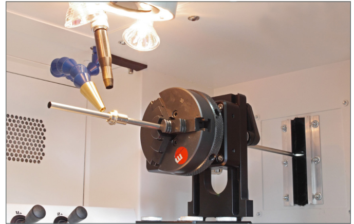
Figure 1. MicroWeld™ enables welding spot diameters as small as 0.1 mm supporting fine welds with minimal peripheral thermal loading.
