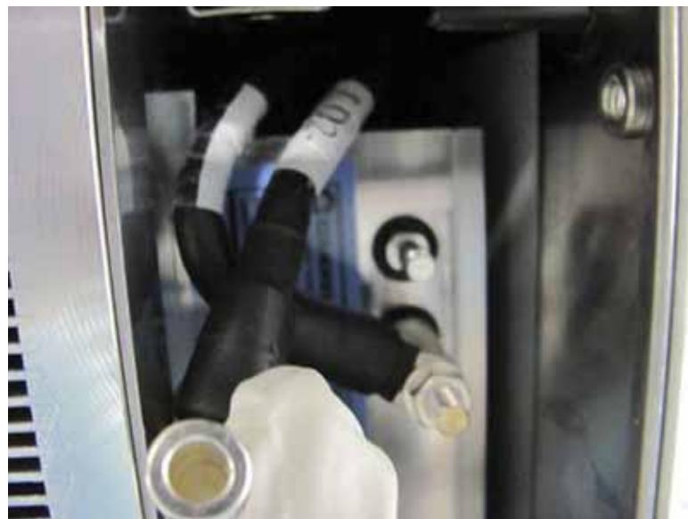
***Figure 3-16. Connect LD2 Voltage Cables***
