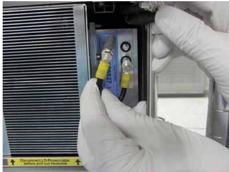
***Figure 3-15. Remove Jumper Cable (or shorting clip) from LD2***
