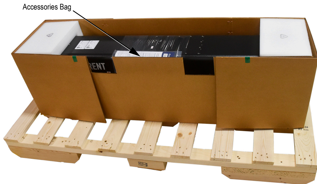
Figure 4-10. Removing the User Documents and Eyebolts
