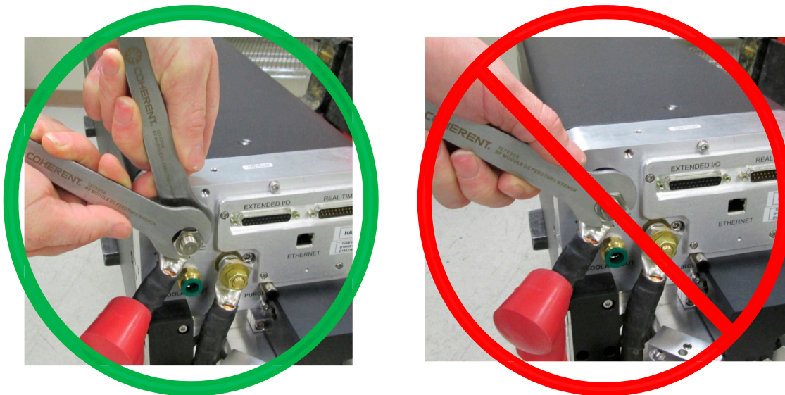
Figure 4-17. +48 VDC Location and Using Two Wrenches
