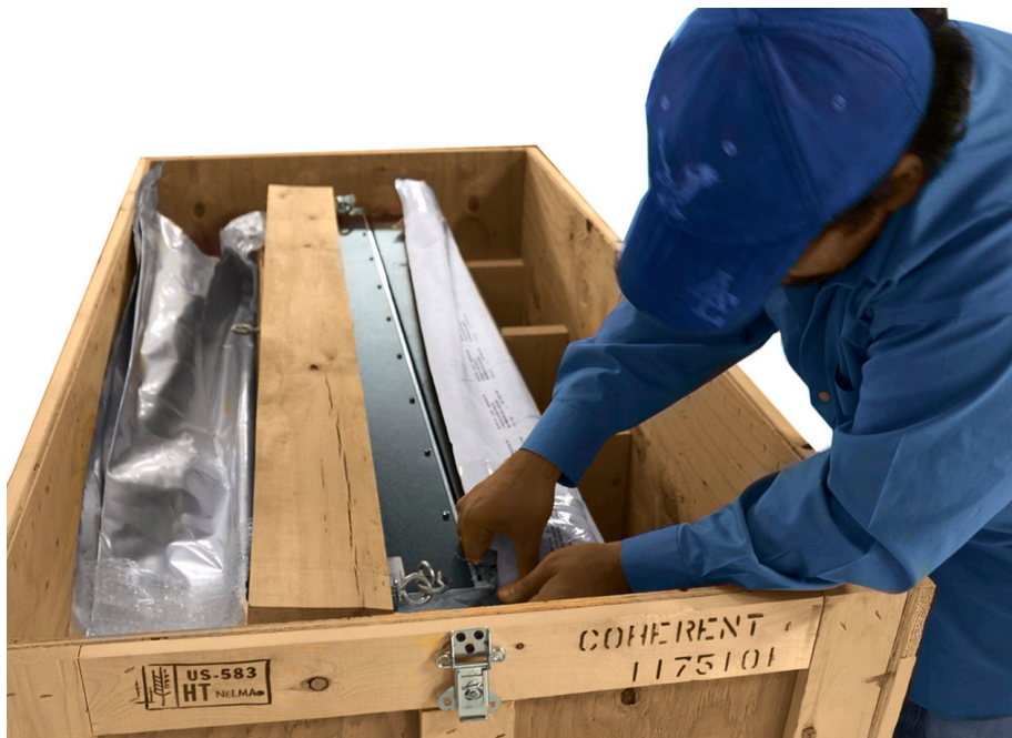
Figure 4-15. Cutting Top of Moisture Seal Bag
