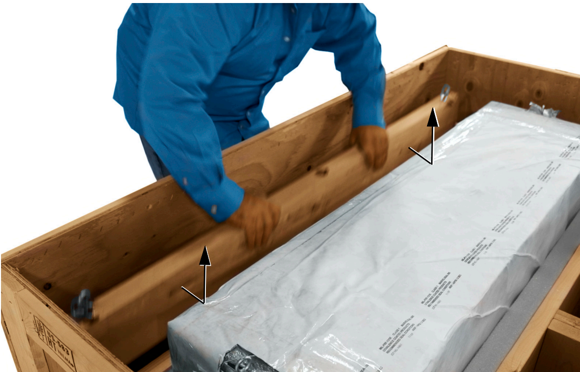
Figure 4-13. Removing Spreader from Crate
