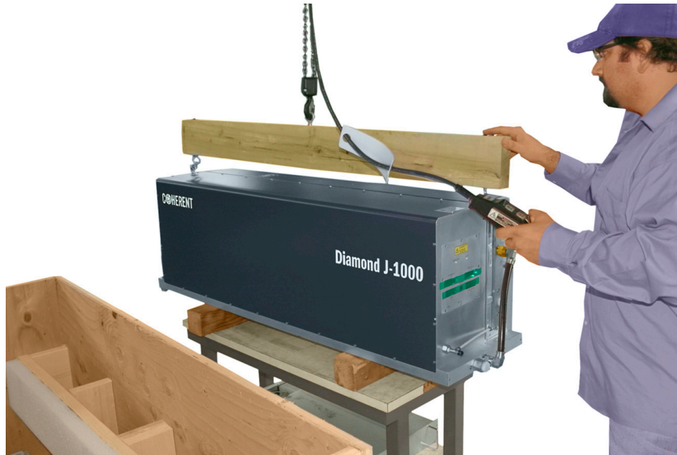
Figure 4-17. Place Laser System on Cart
