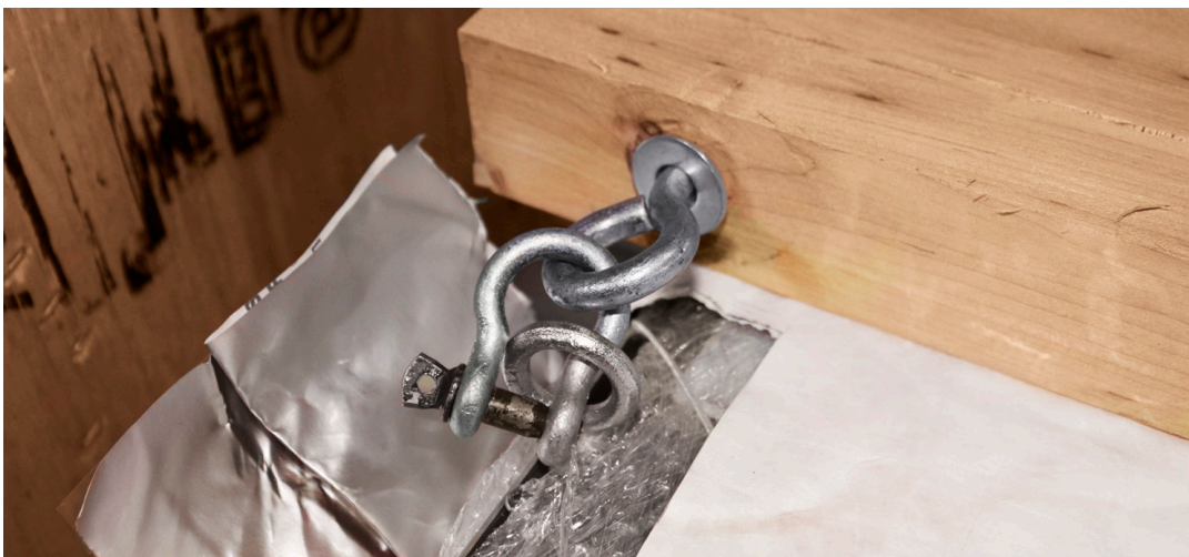
Figure 4-14. Attaching Eye-bolts to Spreader Bar
