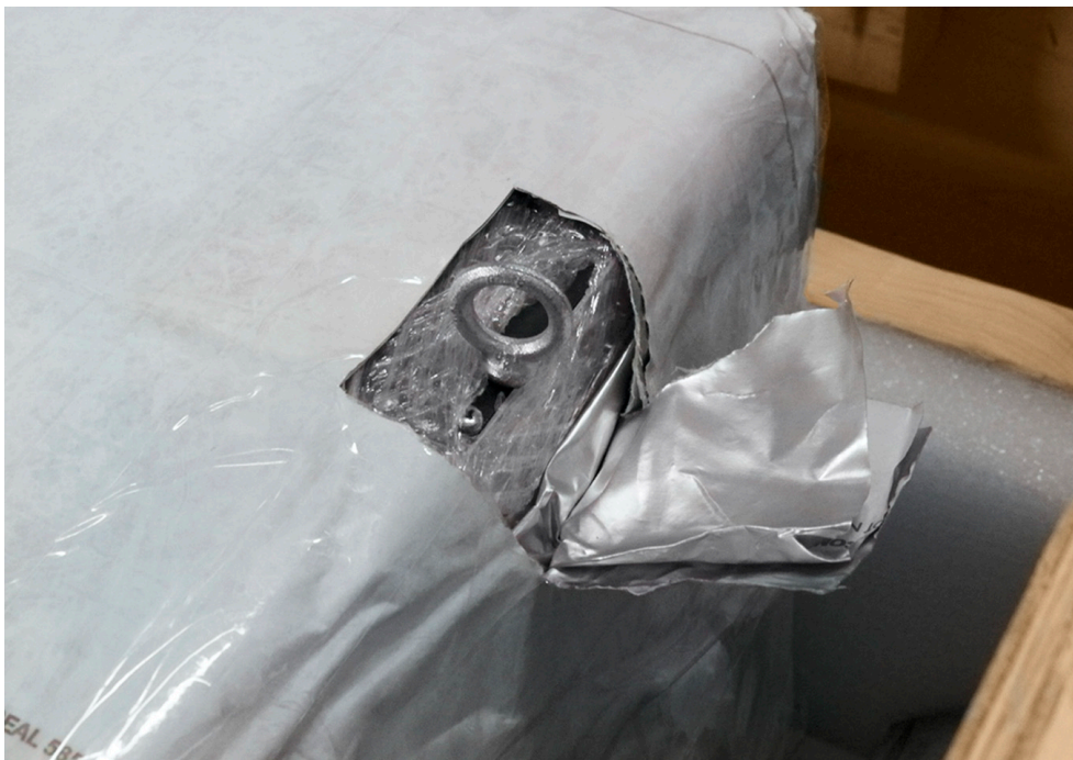
Figure 4-12. Installation of Eye-bolts
