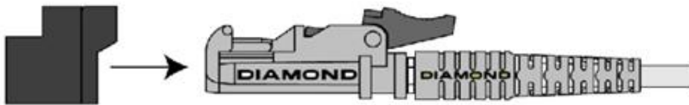
E-2000 Service Adapter 1019034 to hold spring loaded cap open
