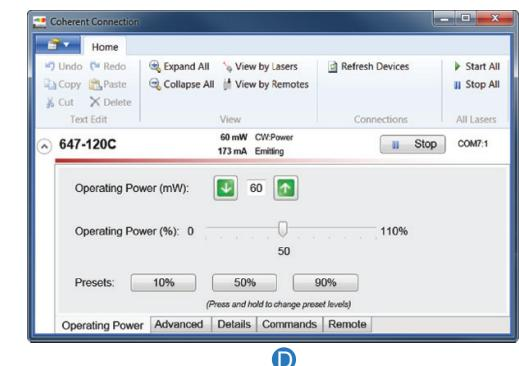
The Coherent Connection Software interfaces to StingRay controller via a USB cable.
