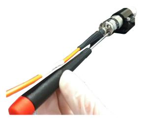
Figure 4-65. Tighten FR Adapter Assembly
