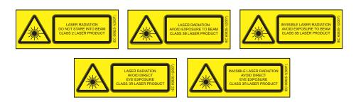
Figure I-3. Example of IEC Warning Labels
