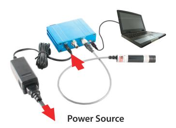
Figure 4-48. Connect Power Supply to Remote
