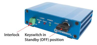
Figure 3-2. StingRay Remote — Interlock and Keyswitch
