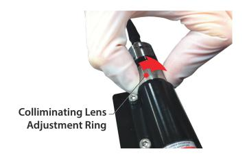
Figure 4-64. Adjust the Collimating Lens
