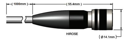
Figure 8-118. Dimensions - Hirose Connector
