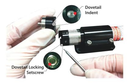
Figure 4-55. Align FR Dovetail Adapter
