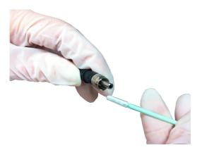
Figure 4-58. Clean the Connector Ferrule
