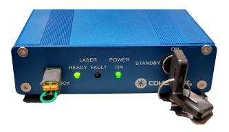
Figure 6-96. LED Indicators - Power to Laser, Keyswitch On, Laser Emits
