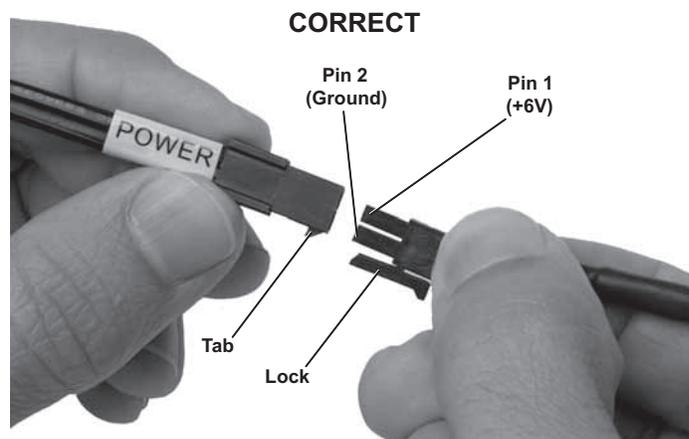
**Figure 3-5. Correct Way to Connect 2-Pin Power Cable**
