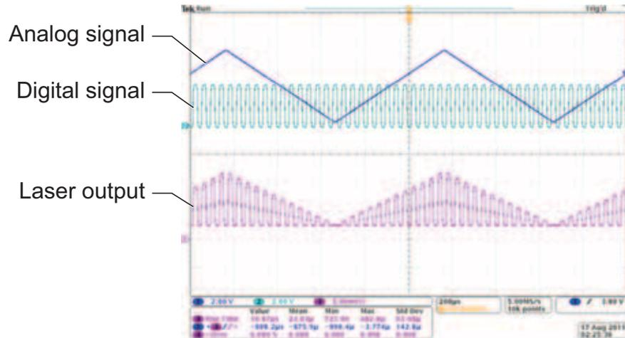
Figure 4-8. Waveforms for Mixed Modulation
