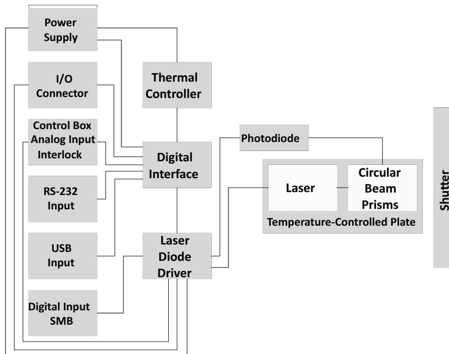
**Figure 2-3. CUBE Laser Head Schematic**
