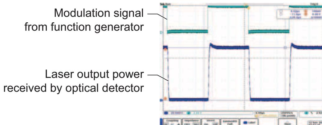
**Figure 4-2. Waveforms for Pulsed Operation (Analog Modulation)**
