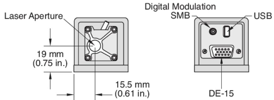
**Figure 2-21. Dimensions — CUBE Laser Head End Views**
