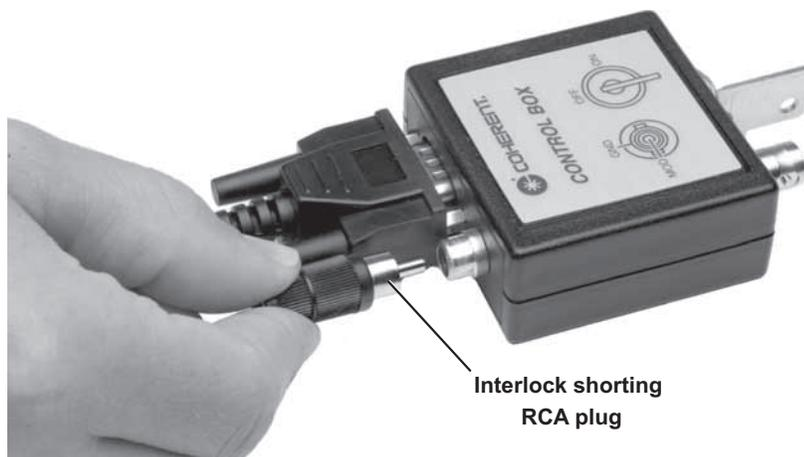
Figure 3-9. Control Box Interlock Connection
