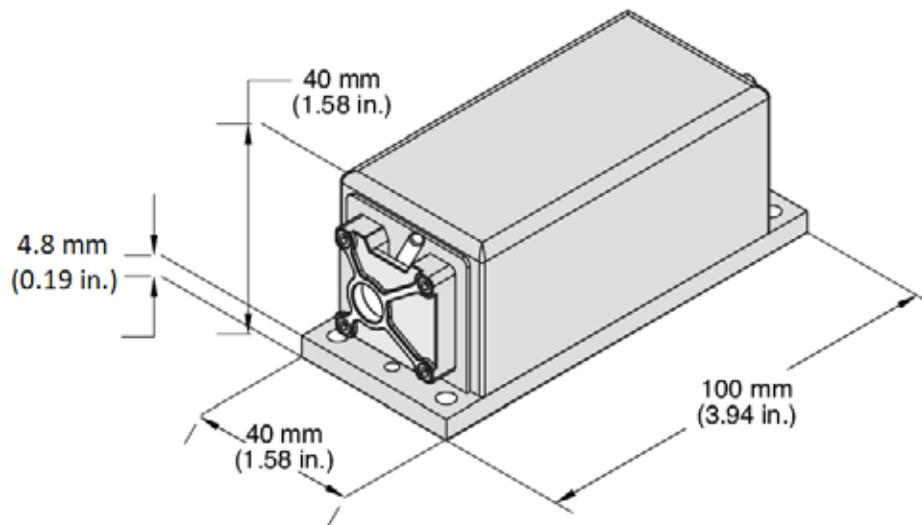
Figure 2-20. Dimensions — CUBE Laser Head
