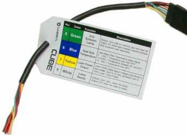
Figure 2-19. CUBE I/O Interface Cable
