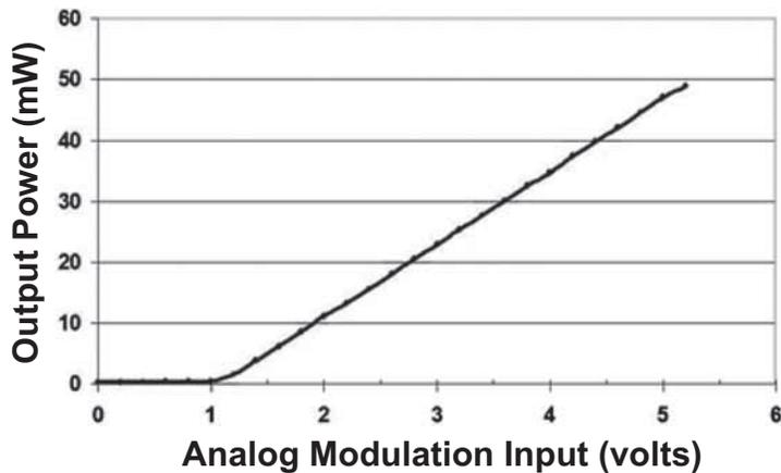
Figure 4-5. Example: CUBE Analog Modulation in Pulse Mode
