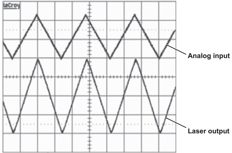
Figure 4-4. Example: CUBE Analog Modulation in Constant Power (CW) Mode
