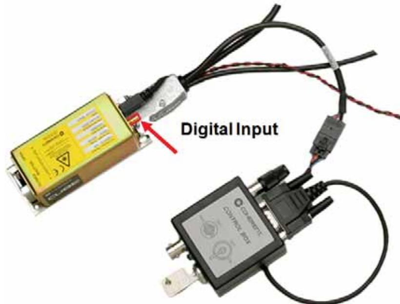
**Figure 4-6. Connection for Digital Modulation**
