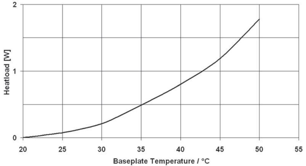
**Figure 2-15. Thermal Dissipation of the CUBE Laser Head**
