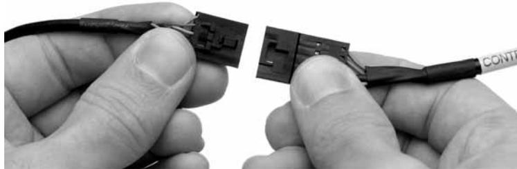
**Figure 3-7. Connect the Control Box**
