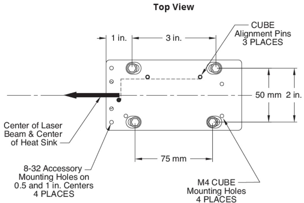
**Figure 2-25. Mounting Holes — Optional CUBE Heat Sink**
