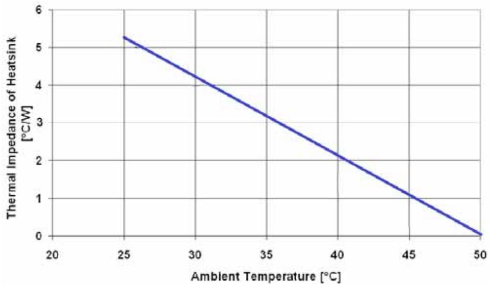
**Figure 2-16. Estimated Heat Sink Requirements for an Ambient Temperature of 50°C**
