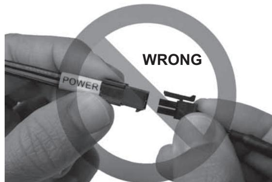
**Figure 3-6. Wrong Way to Connect 2-Pin Power Cable**
