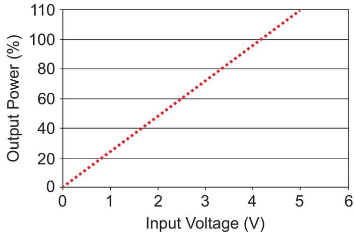
Figure 4-3. Analog Modulation: Power vs. Input Voltage
