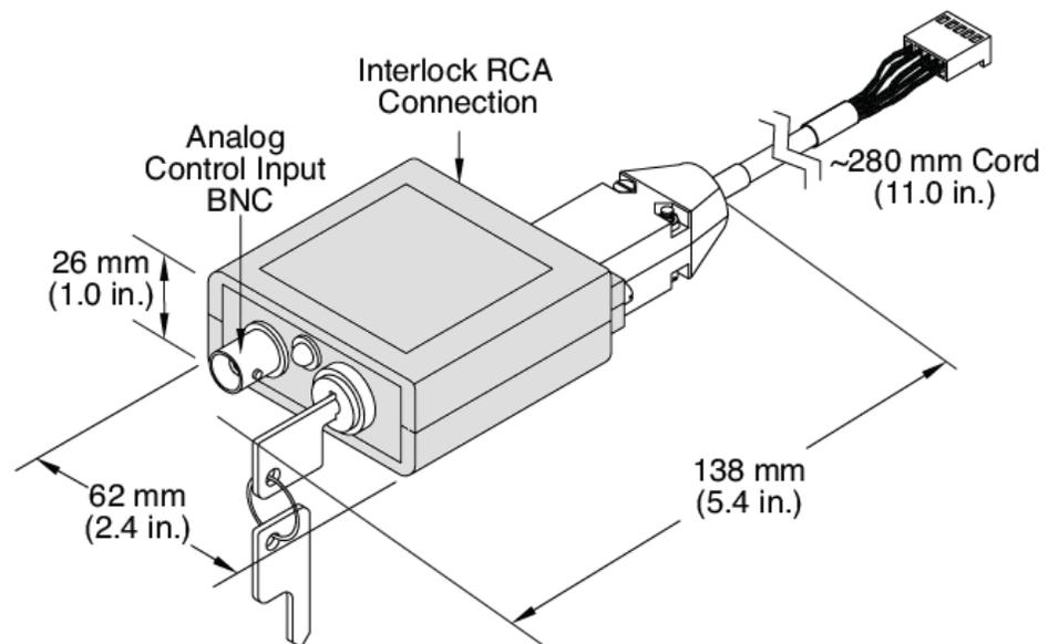
**Figure 2-22. Dimensions — CUBE Control Box**
