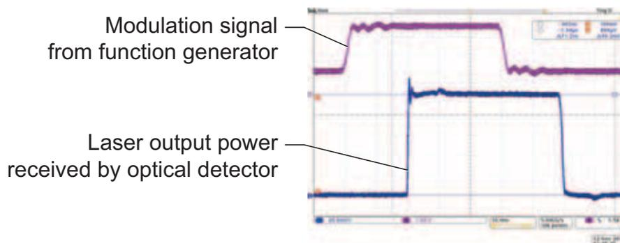
**Figure 4-7. Digital Modulation Timing Diagrams**
