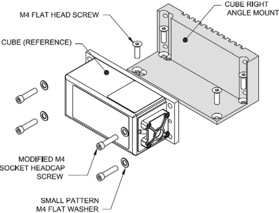
Figure 3-2. Right-Angle Heat Sink Mount Mounting Diagram
