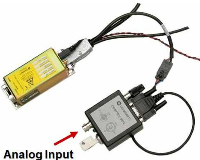
*Figure 4-1. Connection for Analog Modulation*
