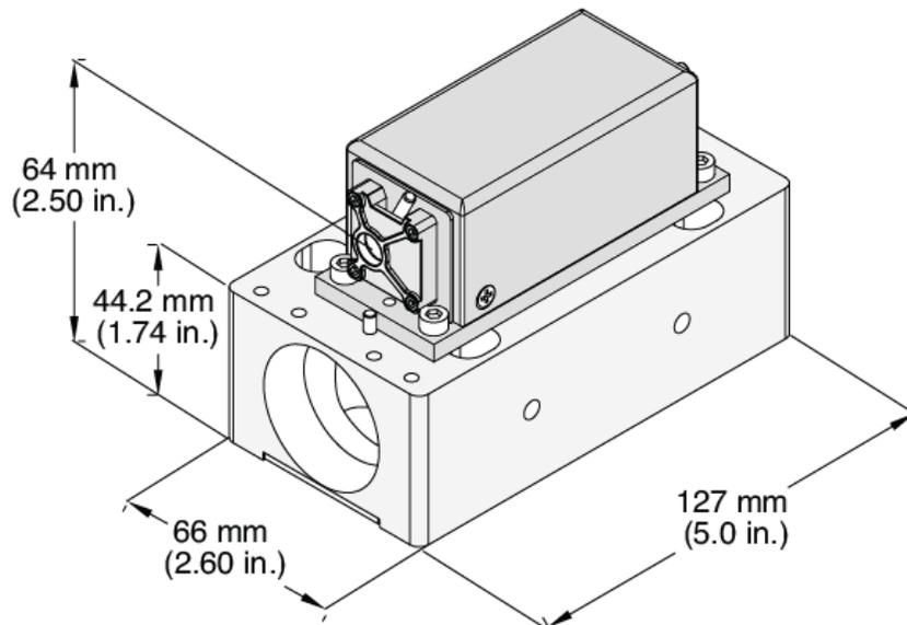
Figure 2-24. Dimensions — Optional CUBE Heat Sink
