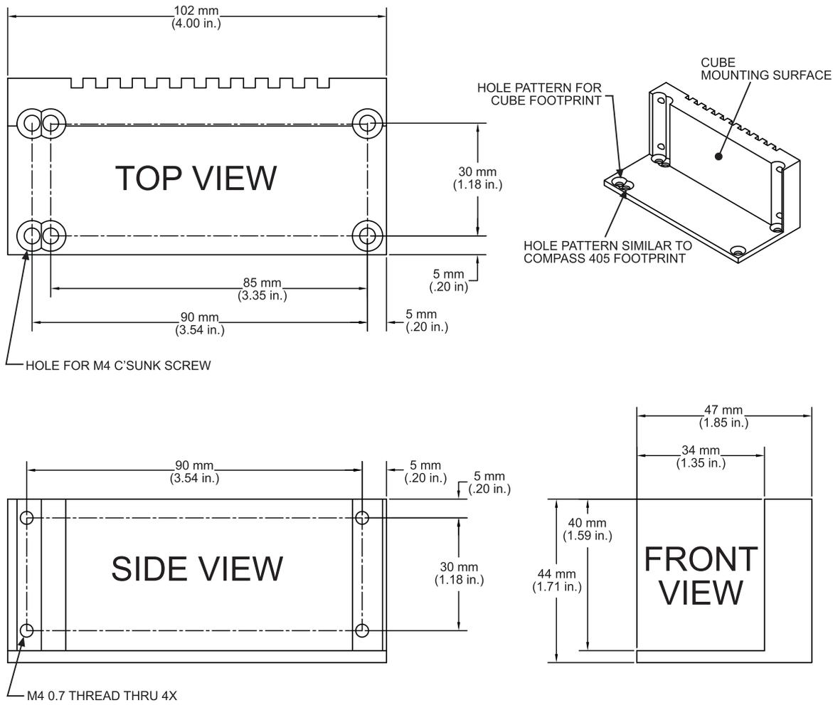
**Figure 2-26. Dimensions: Right-Angle Heat Sink Mount**
