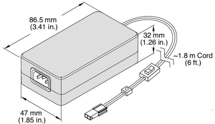
Figure 2-23. Dimensions — CUBE Power Supply
