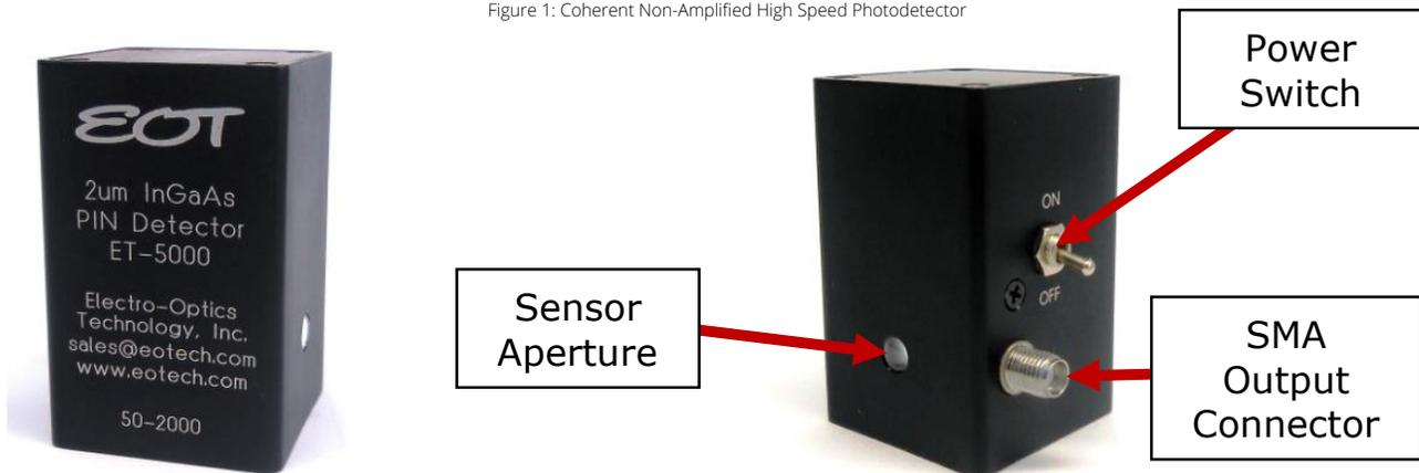
When terminated into 50 Ω into an oscilloscope, the pulsewidth of a laser can be measured. When terminated into a spectrum analyzer, the frequency response of a laser can be measured.
