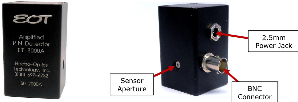
When terminated into 50 Ω into an oscilloscope, the pulsewidth of a laser can be measured. When terminated into a spectrum analyzer, the frequency response of a laser can be measured.
