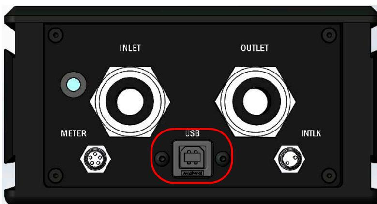
Figure 4-28. PM10K+ USB Connector - USB Model
