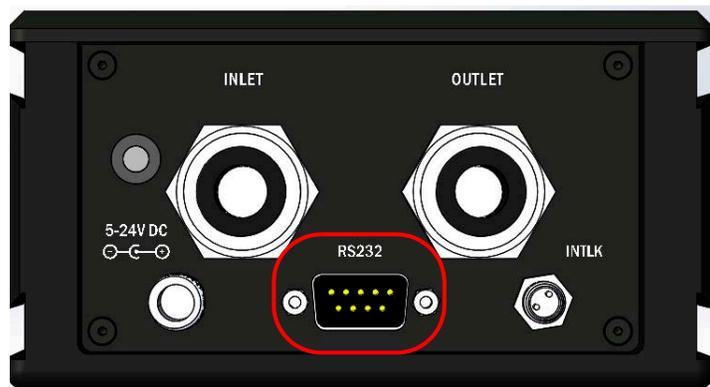
**Figure 4-23. Sensor System RS-232 Port**
