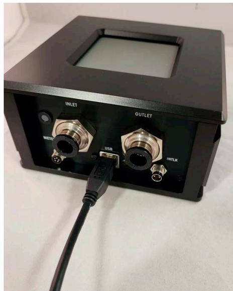
Figure 4-22. Attach USB Cable
