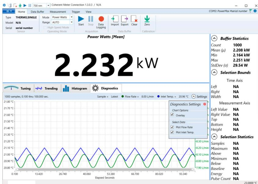
Figure 6-4. Observe Flow Rate and Inlet Temperature
