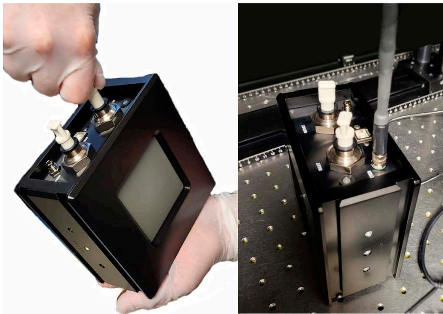
Figure 9-6. Install Protective Caps
