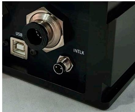
**Figure 3-16. M8, 2-pin Barrel Connector for Interlock**
