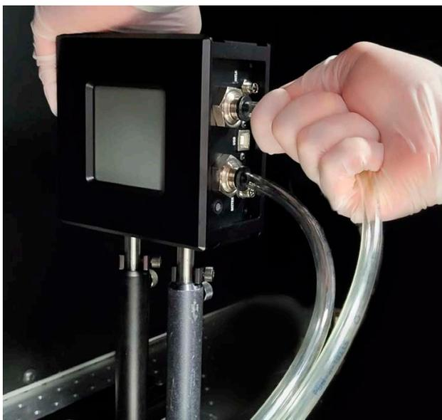
**Figure 4-16. Attach Water Hoses to Fittings on Sensor**
