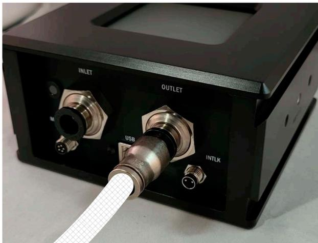
**Figure 4-20. Insert Hose, with Adapter, into Fitting on Sensor**
