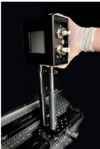
**Figure 9-4. Remove Sensor from Mount (Post-mount setup)**
