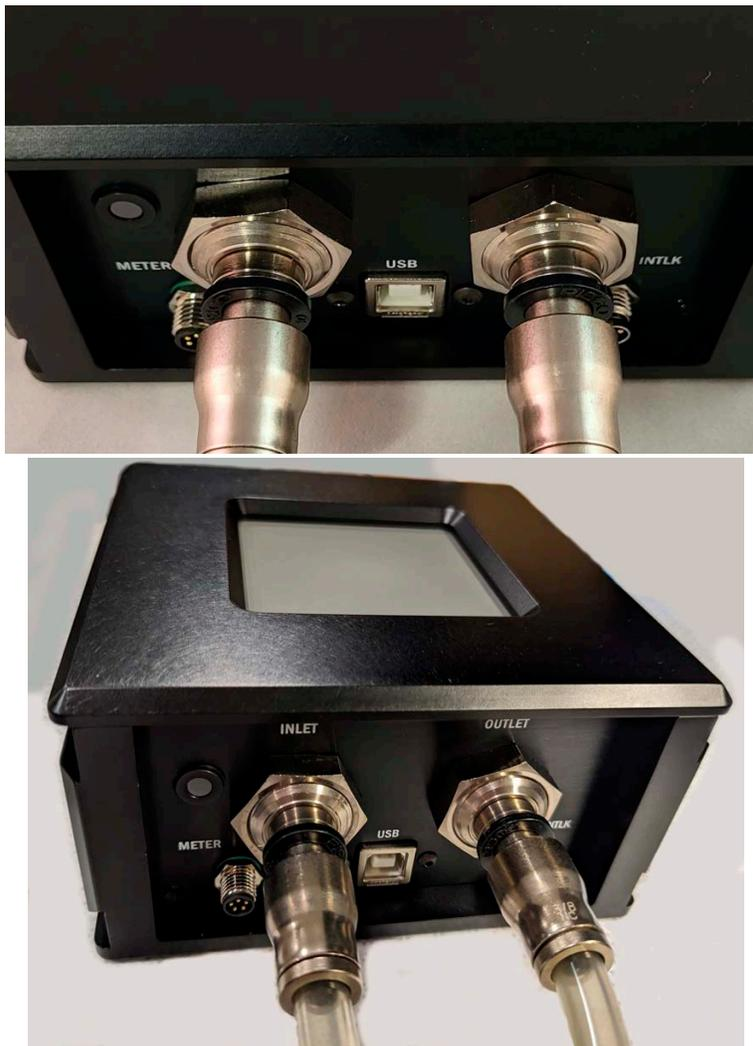
**Figure 4-21. 3/8-in Hoses with Adapters Installed**
