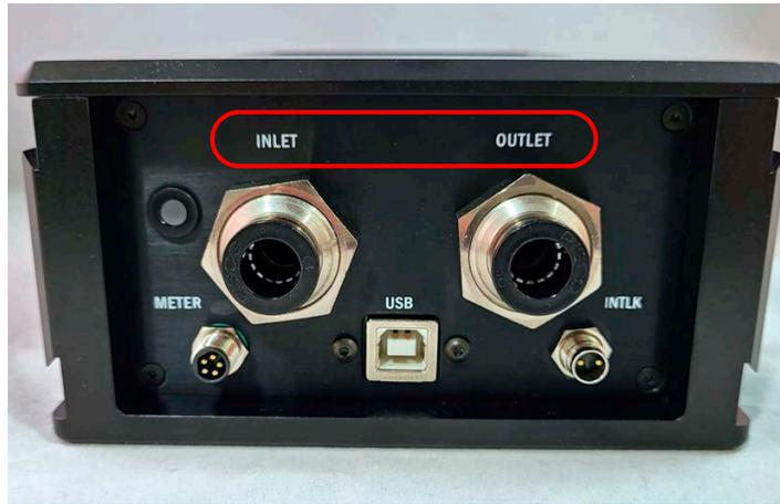
**Figure 4-17. Water Inlet and Outlet Fitting Labels**
