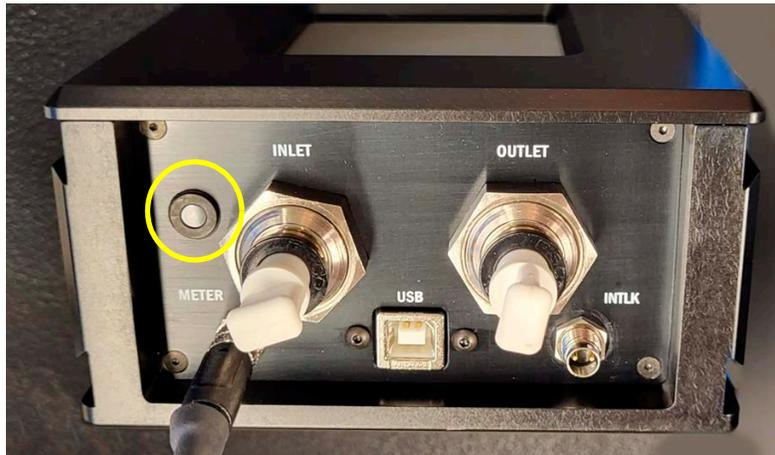
**Figure 5-1. LED Indicator Light Location**
