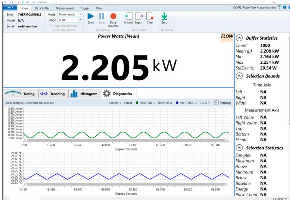
Figure 6-3. Water Flow Rate and Temperature in Diagnostics Tab
