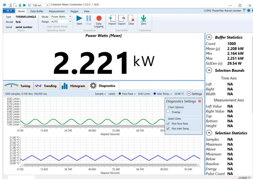
Figure 7-5. Diagnostics Tab - Temperatures and Water Flow
