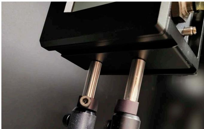
Figure 4-13. Bottom 1/4-in. Mount Setup Example
