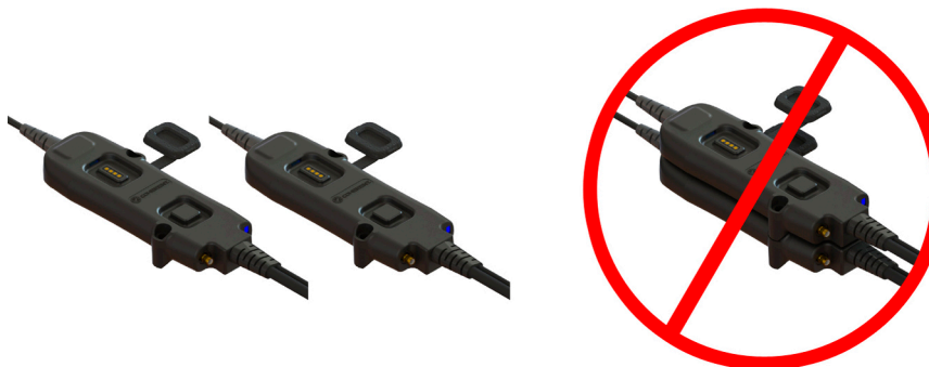
Figure 3-7. Make Sure That Sensors are NOT Stacked
