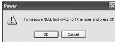
The system now measures the ambient light level. Clicking the OK button will cause the software to subtract the measured level from the subsequent measurements.
