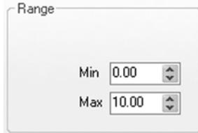
The Power Range magnifies the beam power display. The needle graph display is affected accordingly.
