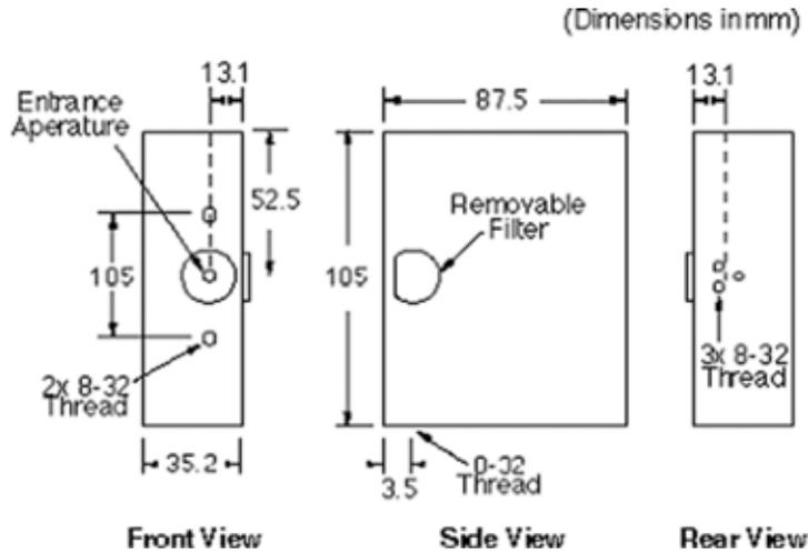
Figure 5-2. BM-3 Silicon Detector Head Dimensions
