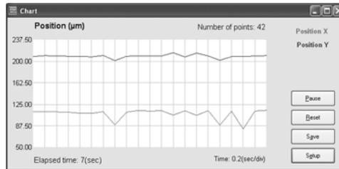
The Width/Position Chart window provides a real-time strip chart display of beam position (X, Y) versus time, or beam width of V and W profiles measured at the System Clip Level.
