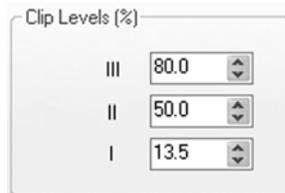
The three clip levels determine the levels at which the width of V and W profiles are to be measured by the BeamMaster-USB system.
