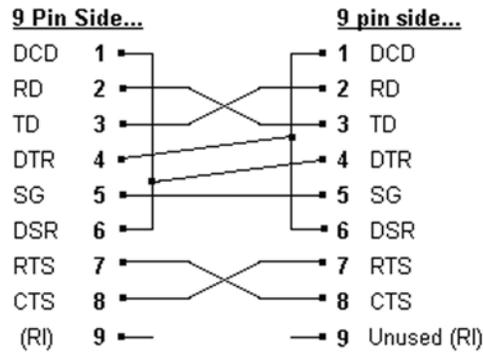
Figure 4-3. Null-Modem with 9 Pins on Both Sides
