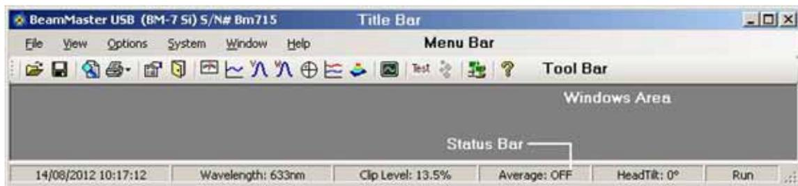
**Figure 3-1. BeamMaster-USB Window Interface—Main Elements**
