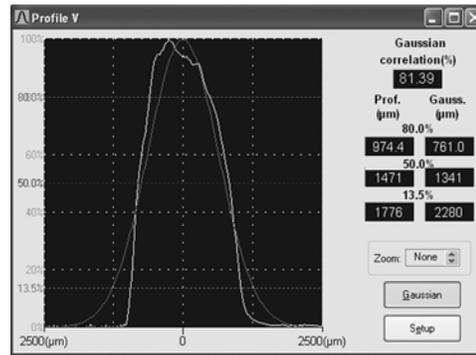
This function determines how closely the measured beam profile matches a theoretical Gaussian profile. When the Gaussian button is activated, a Gaussian profile is overlaid on top of the current measured profile in real time. The gaussian fit profile is in red.
