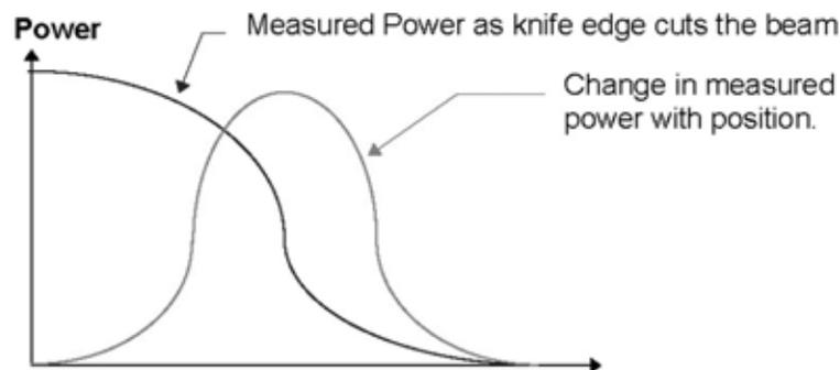
The analog power reading is digitized with a high speed A/D (Analog-to-Digital) converter. At the same time, the exact position of the knife-edge is monitored so that beam width information can be determined. The beam profile for each knife-edge is then obtained in software by taking the derivative of the measured power curve. The beam profile is perpendicular to the knife-edge and each
