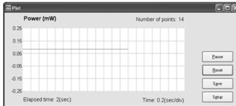
The Plot window provides a graphical display of beam power versus time. The graph presentation includes the temporal power fluctuations and provides a way to observe long-term power fluctuations. The Plot window also displays the number of points accumulated, elapsed time clock, and the exact time/division partition.
