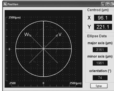
The Position function provides a real-time display of the beam centroid position, as well as a beam foot print. This window can be used to align the detector head with the incoming laser beam. Settings can also be customized by clicking the Setup button.
