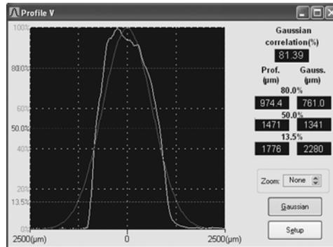
The Profile Window graphically displays details of the beam's intensity profile along the V axis. In addition to the profile information, there is a display of beam width at three different clip levels. The clip levels (80%, 50%, and 13.5%) may be changed using the Setup button.
