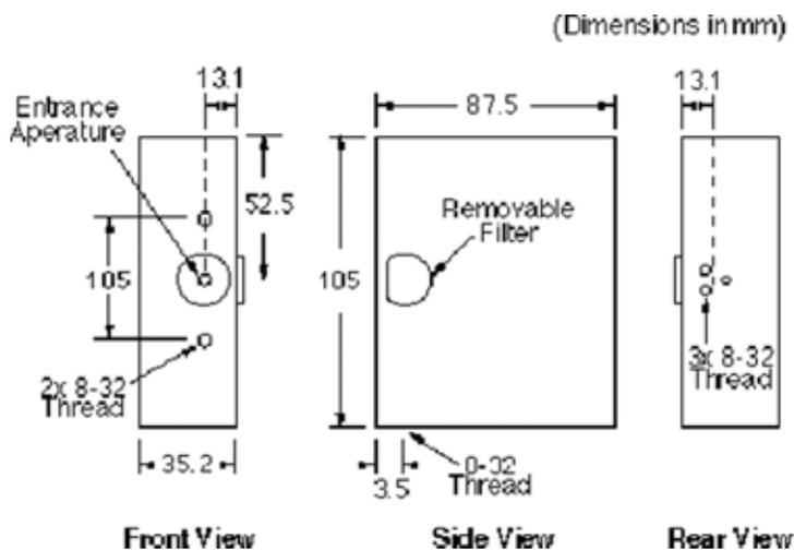
**Figure 5-1. BM-3 InGaAs Detector Head Dimensions**
