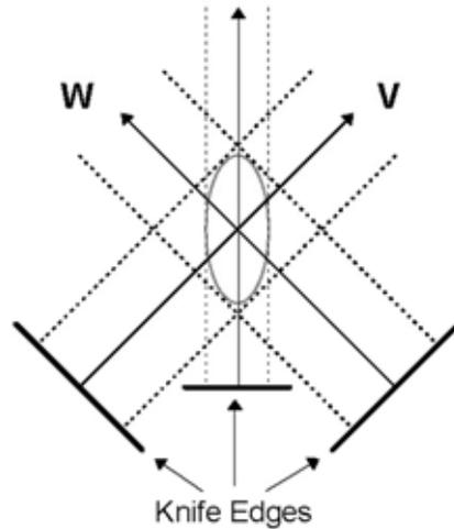
There are two primary knife-edges used for the main profile display. These knife-edges generate profile—referred to as W and V—that are set perpendicular to each other and are oriented at 45 degrees in relation to the base of the head. These profiles are used to provide beam width, position, and gaussian fit analysis. The other knife-edges are used for reconstructive tomography.
