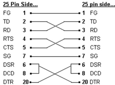
*Figure 4-1. Null-Modem with 25 Pins on Both Sides*
