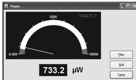
The Power selection activates the power meter display window. The display shows real-time power as a needle graph or a digital value. Several buttons provide easy and quick control of the Power functionality.
