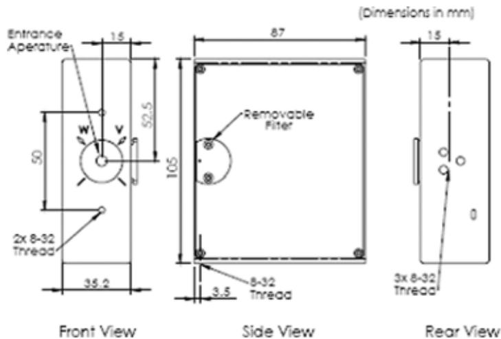
Figure 5-4. BM-3\* InGaAs Detector Head Dimensions
