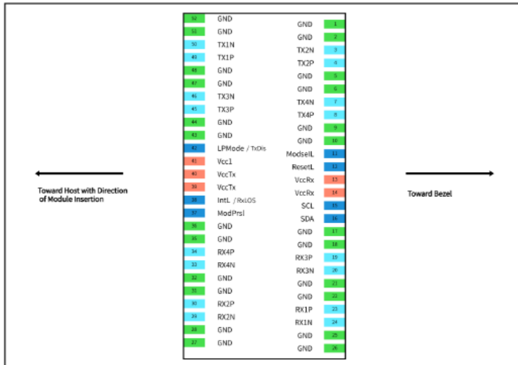
Figure 2 QSFP112 Host PCB pad assignment
