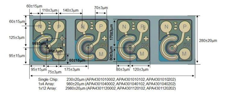
N: n-contact (common cathode) P: p-contact (anode) M: mechanical pad
