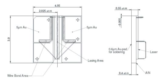
Soldering recommendation: T max=250 °C , Time max =1 min, no flux
