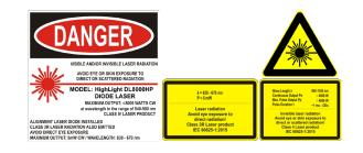
Coherent-Dilas industrial lasers are designed in strict accordance with the respective safety regulations. We certify that each laser manufactured by our company complies with FDA Radiation Performance Standards, 21 CFR Subchapter J and with IEC 60825. Warning labels as shown in the figure appear on each Coherent-Rofin laser to indicate the respective classification.
