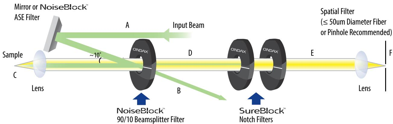
A high throughput low frequency Raman spectroscopy system can be assembled by combining a NoiseBlock 90/10 beamsplitter with two SureBlock notch filters and optional NoiseBlock ASE suppression filters. The resultant system is capable of measuring Raman signals as low as  $<10\text{cm}^{-1}$  from the laser line.
