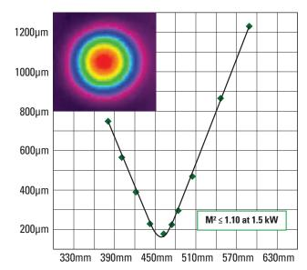
Beam quality,  $M^2$  , achieved with a 0.06 NA, 25/400  $\mu m$  , Yb-fiber with M+ specifications operating at an output power of 1500 watts.
