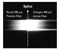
By optimizing the core sizes and NA, and specifying the MFD, M+ fibers have better matched MFD's for improved splice performance.
