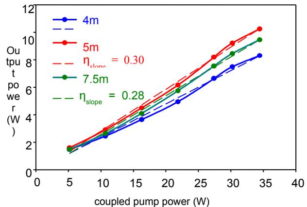
Figure 1: Slope efficiency of a 10m long PM-LMA-EYDF-25/300 CW fiber amplifier pumped at 975nm and seeded with 100mW at 1559nm (left) and Slope efficiency of a 500ns seeded amplifier as a function of coupled pump power for 4m, 5m and 7.5m fiber (right).
