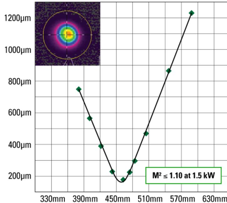
Beam quality,  $M^2$ , achieved with a 0.06 NA, 25/400  $\mu\text{m}$ , Yb-fiber operating at an output power of 1500 watts. Lower NA LMA fibers deliver excellent beam quality at the highest powers.
