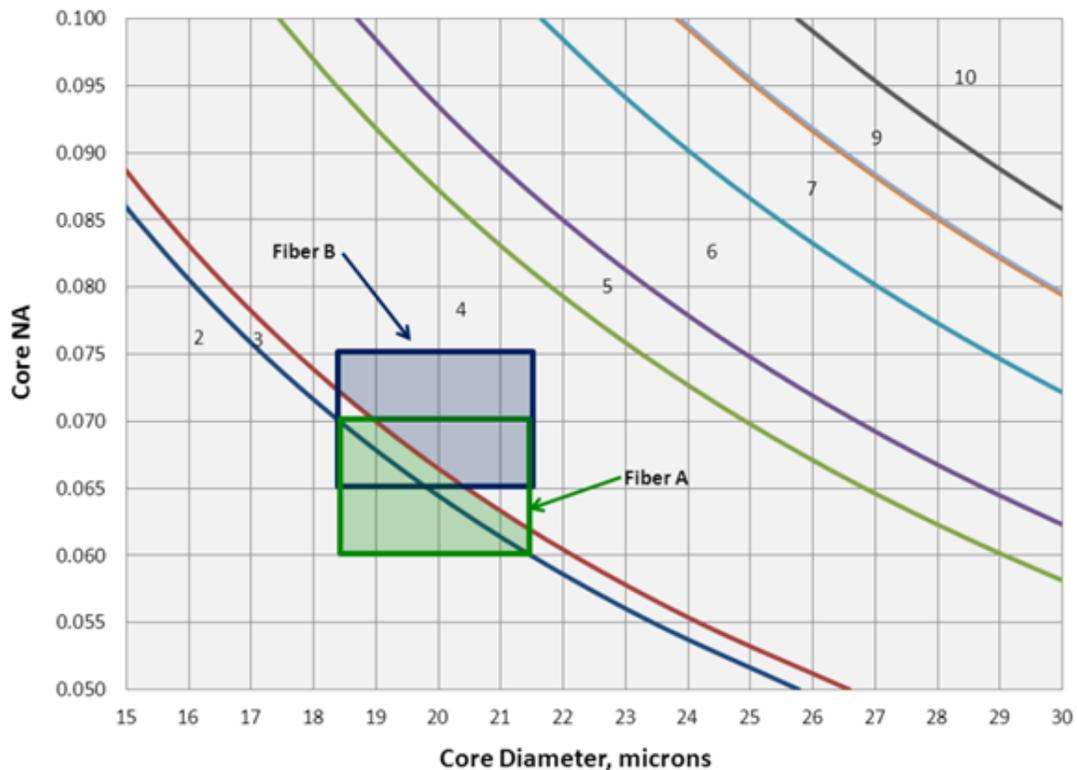
*Number of linearly polarized modes supported by fibers with different core sizes and NAs operating at 1064 nm. Lower NA fiber offers the largest operating range of fewest modes making it ideally suited for high powers while maintaining beam quality and fiber reliability.*
