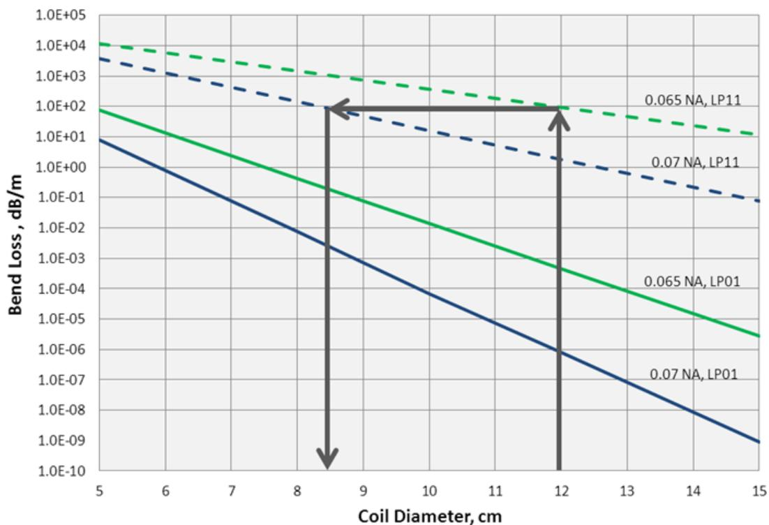
*LP01 and LP11 bend losses of 20  $\mu\text{m}$  core diameter fibers at 1060 nm vs. coil diameter for 0.065 NA (in green) fiber and 0.07 NA (in blue) fiber. The 0.065 NA fiber has greater HOM bend loss enabling users to more easily discriminate the fundamental (LP01) mode from the HOMs making it easier to design fiber lasers with diffraction limited beam quality.*
