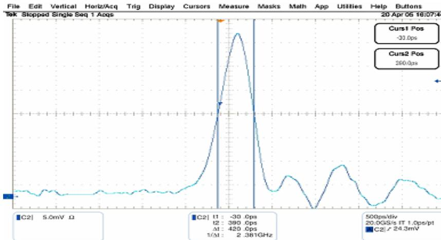
**Figure 8:** Output pulse measured with a 2.5GHz oscilloscope with a 120ps rise time and a Newport AD300 amplified InGaAs detector. The GenII LFM was producing 10W of average power and a peak power in excess of 2MW.
