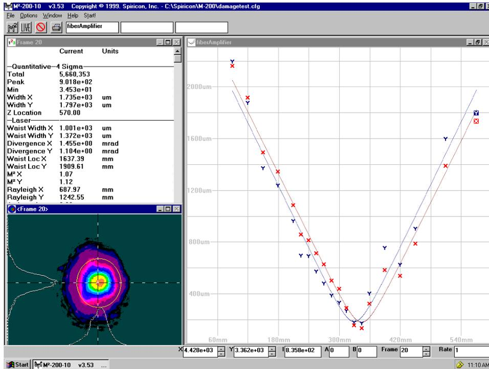
Figure 9:  $M^2 < 1.15$  measurement at 10W of average power.
