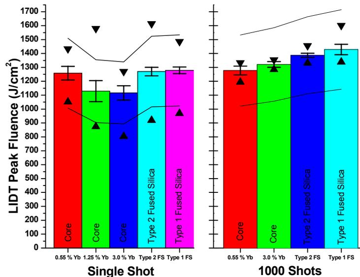
**Figure 1:** Single and 1000 shot summarized LIDT results of the Yb doped cores and the two types of fused silica. Minimum and maximum LIDT are displayed by triangles pointing up and down respectively. The  $\pm 20\%$  experimental error is shown by the solid black lines.
