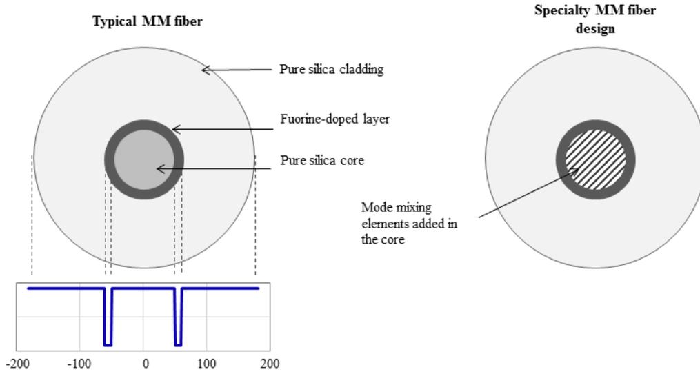
Fig. 6: Schematic of typical MM process fiber with 100  $\mu\text{m}$  core and 0.22 NA (left) and of the specialty MM fiber for beam control (right).
