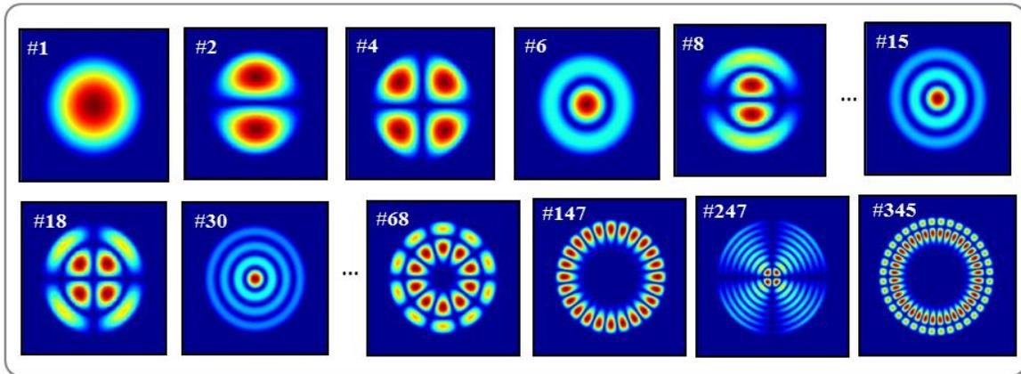
Fig. 1: Intensity profile of a few of the transverse modes available in the core of multimode step-index circular core fibers.
