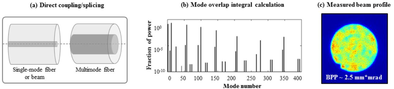
Fig. 3: (a) Schematic of the direct coupling between the SM and the MM fibers. (b) Calculation results of the mode overlap integral. (c) Profile of the beam measured at the MM fiber output (100  $\mu\text{m}$  core, 0.22 NA) when the SM fiber is directly spliced.
