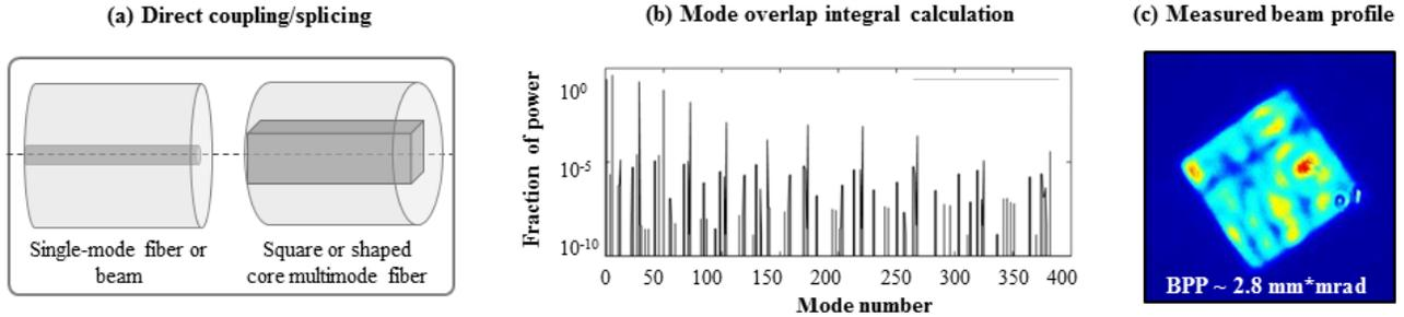
Fig. 5: (a) Schematic of the direct coupling between the SM and the MM shaped-core fibers. (b) Calculation results of the mode overlap integral. (c) Profile of the beam measured at the MM square-core fiber output (100  $\mu\text{m}$  core, 0.22 NA) when the SM fiber is directly spliced.
