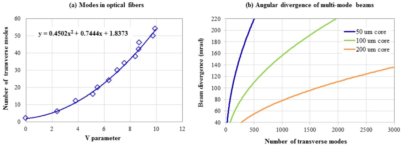
Fig. 2: (a) Number of modes available in a MM fiber as function of the V parameter. (b) Calculation of the beam divergence as function of the order of the HOM excited in the MM fibers. Results are shown for 50, 100 and 200  $\mu\text{m}$  core diameter fiber with 0.22 NA.
