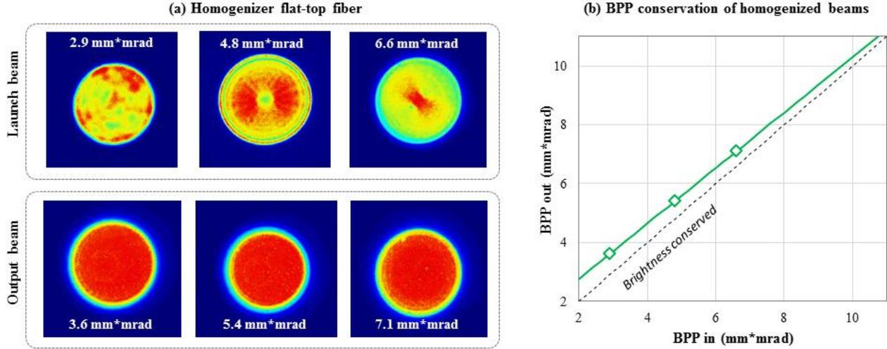
Fig. 11: (a) Experimental demonstration of the homogenizer capabilities of the flat-top fiber design for a variety of MM input beams. (b) Plot of the BPP measured at the output of the specialty flat-top fiber as function of the BPP of the launched beam. Measurements shown with the green markers are compared against the ideal case of BPP conservation (dashed line), i.e. brightness conservation. Both launch fiber and flat-top fiber cores were 100  $\mu\text{m}$  in diameter.
