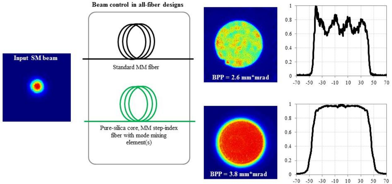
Fig. 9: Measurement of the beam properties, including 2D and 1D beam profiles and angular beam divergence emerging from standard MM fiber (top) and from the specialty flat-top MM fiber (bottom) when a SM beam is launched using conventional splicing or coupling techniques.
