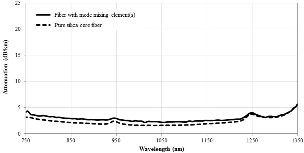
Fig. 8: Measured core attenuation compared between a standard MM fiber and the same fiber with mode mixing elements in the core. Both fiber core diameters are 100  $\mu\text{m}$ .
