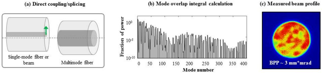
Fig. 4: (a) Schematic of the offset coupling between the SM and the MM fibers. (b) Calculation results of the mode overlap integral. (c) Profile of the beam measured at the MM fiber output (100  $\mu\text{m}$  core, 0.22 NA) when the SM fiber is offset spliced.
