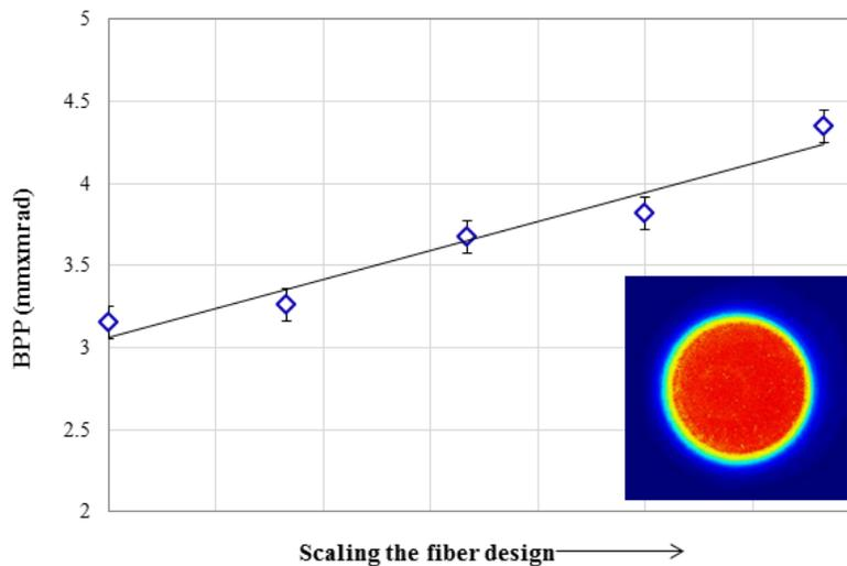
Fig. 10: Measured BPP emerging the specialty flat-top fiber as one design parameter of the mode mixing element(s) is tuned. As the BPP increases linearly, the beam profile maintains a uniform flat-top shape.
