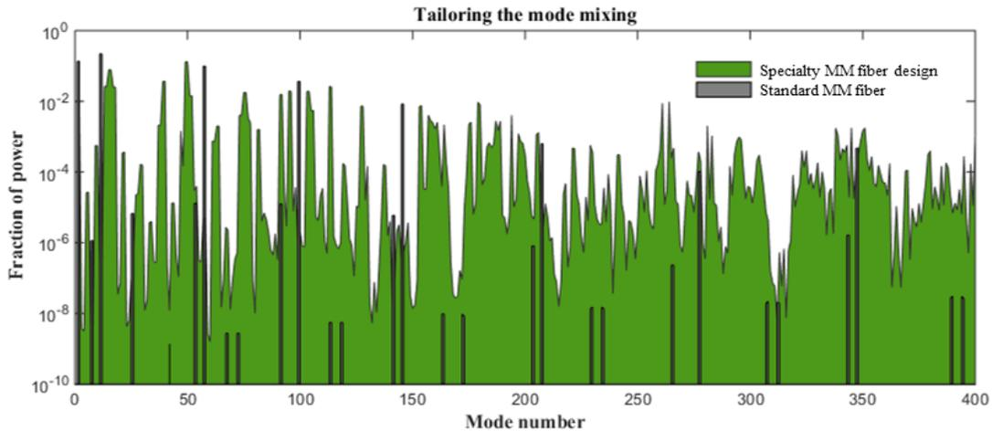
Fig. 7: Mode overlap calculations showing the mode mixing in a standard MM fiber (black) and in the specialty fiber design (green) in the case of an incident SM beam.
