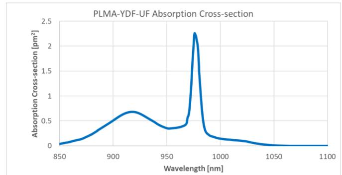
Figure 1: PLMA-YDF-UF absorption cross-section.
