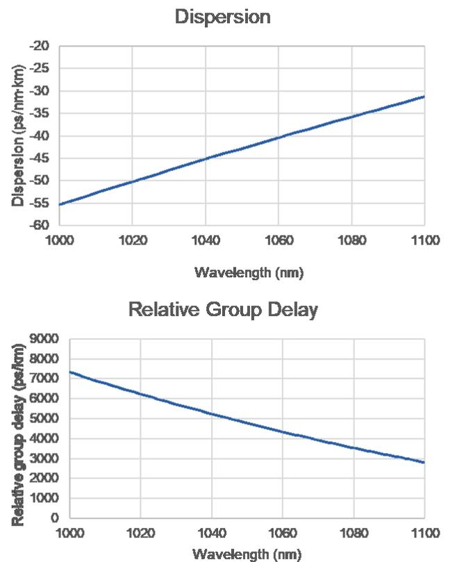
Figure 3: PLMA-YDF-14/125-UF Dispersion (top) and RGD (bottom).
