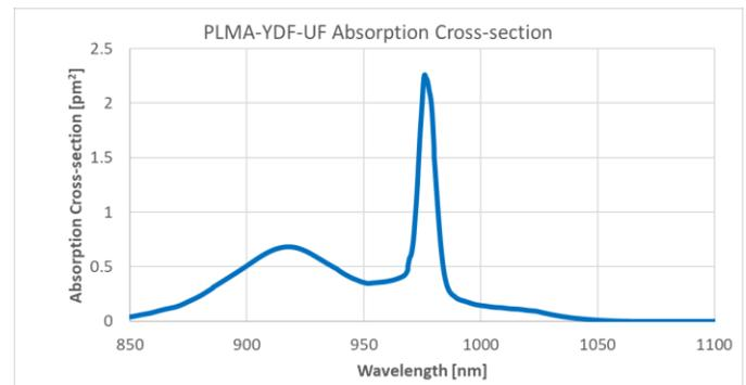
Figure 1: PLMA-YDF-UF absorption cross-section.
