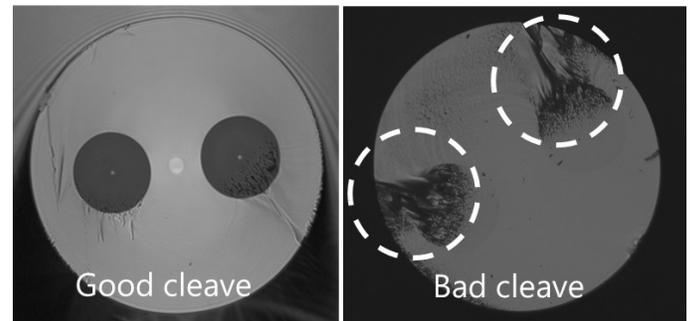
Figure 2: Example of good cleave (left) and bad cleave (right).
