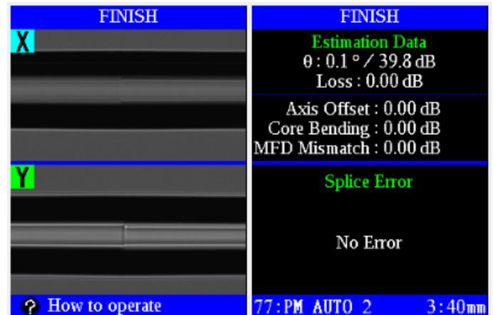
Figure 3: Optimized splice with minimal heat distortion and low loss.
