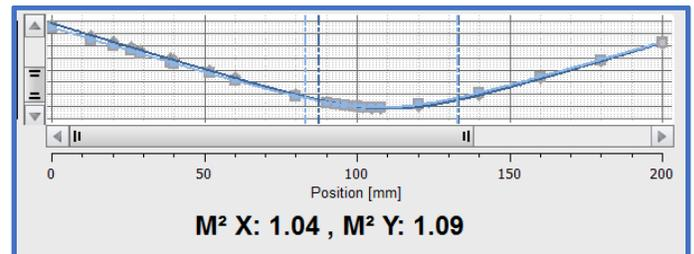
Figure 2: PLMA-YDF-14/125-UF M<sup>2</sup>.
