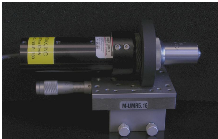
Figure 4: free space module secured in a threaded adapter
