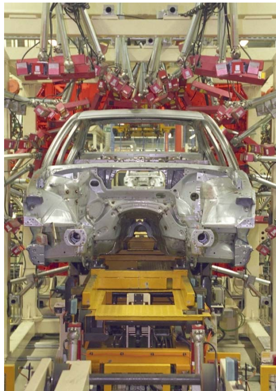
Figure 3. The contemporary automotive production line features an extremely high level of automation, including robotic actuators and supporting machine vision systems.
