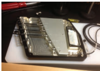
Figure 2. The OBIS Galaxy (shown with the top cover removed) allows plug-and-play combining of up to eight separate fiber coupled lasers into a single output fiber. Courtesy of Sam Lord.
