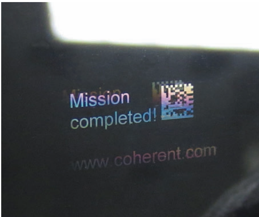
Figure 3. Color mark on glass, produced using a 700-ps laser (Coherent, Helios) operating at 532 nm.
