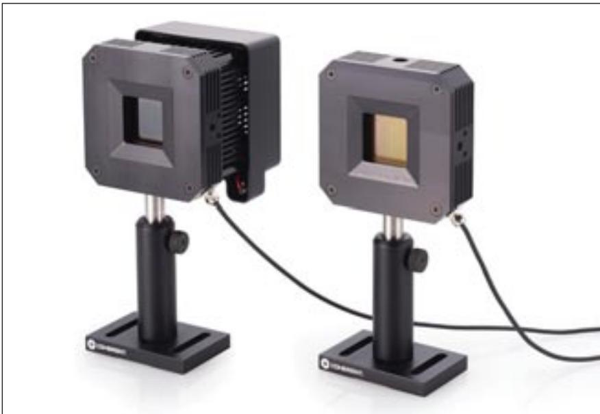
Figure 5. Thin film thermoelectric sensors are available with a broadband coating, which operates from 300 nm to 11  $\mu$ m, and a higher damage threshold (up to 14 kW/cm<sup>2</sup>) coating, which covers both 355 nm to 1100 nm and 9  $\mu$ m to 11  $\mu$ m.
