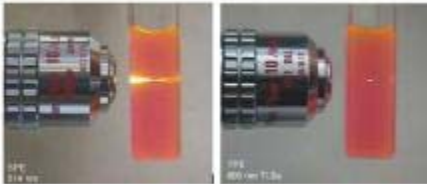
Fig. 1: Multiphoton microscopy provides inherent three-dimensional resolution. With conventional (single photon) excitation of samples, fluorescence is excited along the entire beam path. With multiphoton absorption, fluorescence is only excited by the high intensity at the beam waist.
