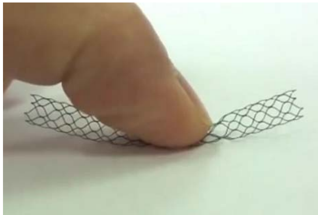
Heart valve scaffolds are laser cut from a nitinol tube blank. Image courtesy of STI Laser Industries.
