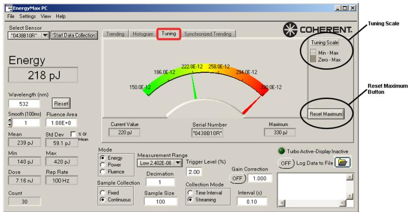
**Figure 6. An analog needle style display is included to facilitate laser and optics adjustment.**
