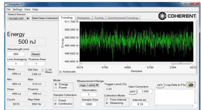
**Figure 4.** The operating mode and data collection parameters for the sensor are chosen on the main screen, and acquired data can be viewed in various ways, such as a plot of energy vs. time.
