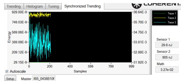
**Figure 2** Multiple EnergyMax units can be stacked to enable ratiometry (above), and system software enables data from multiple channels to be monitored.
