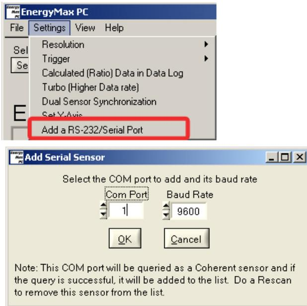
**Figure 3.** Connecting with an EnergyMax-RS sensor simply requires selecting the “Add a RS-232/Serial Port” option from the Settings menu, and then specifying a Com Port.
