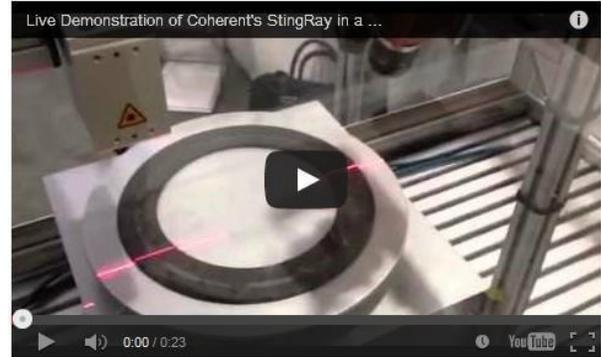
In this relatively simple application, a single line projection spans the diameter of the clutch plate as it is rotated. Triangulation of the red line image then provides a high resolution scan of the entire plate.
