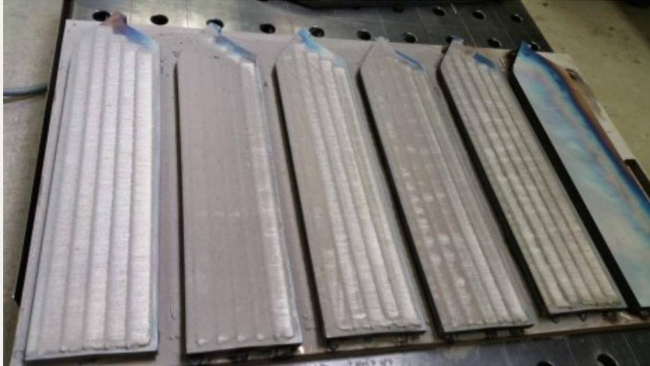
*Cladding makes fan blades more durable, but it is important that the process does not induce distortion, otherwise expensive rework will be required.*
