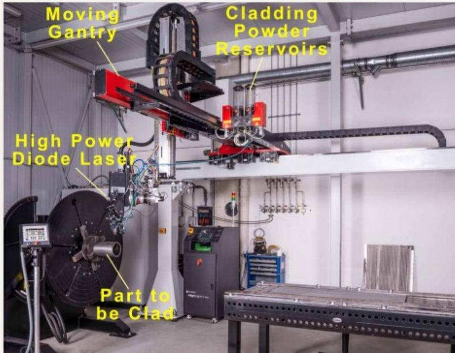
*In the laser cladding system developed at Castolin Eutectic International, a Coherent HighLight 10000D is mounted on a large gantry, enabling cladding of parts up to 5m in length.*
