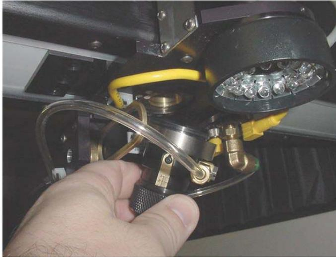
**Figure 2.** Nozzle Assembly Removal
