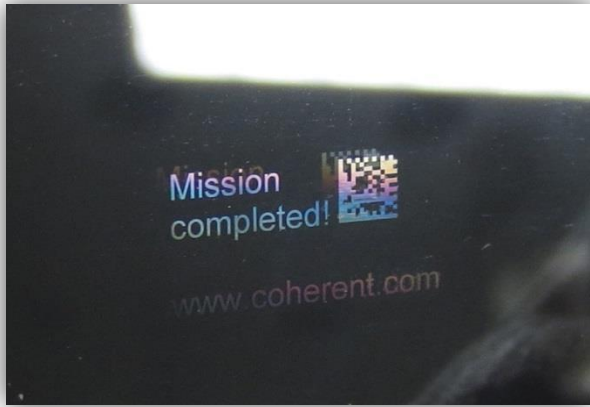
Figure 2: Color mark on glass, produced using a Helios laser operating at 532 nm.
