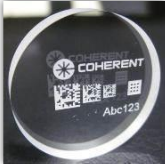
Figure 3: Picosecond lasers can be used to mark sapphire, which is difficult to mark by other means due to its extreme hardness.
