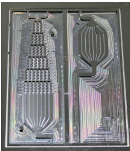
Detail of microfluidic mold insert. Left half shows a mixer and reaction area for two fluids, while the right half depicts an extended flat chamber for interaction of fluid constituents with light. Courtesy of Kugler GmbH.
