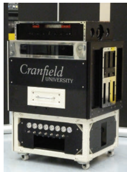
Micro-4 Machining from Loxham Precision Ltd., a ‘micro-factory’ precision machining center (Centre for Innovative Manufacturing in Ultra Precision). Courtesy of the Centre for Innovative Manufacturing in Ultra Precision and Cranfield University.
