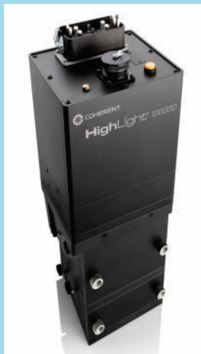
Figure 2. Existing high-power direct diode laser systems are exemplified by the Coherent HighLight 10000D. Its 10-kW output with variable beam profile can be specifically optimized for large area and high deposition rate cladding.
