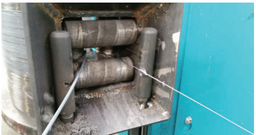
Figure 4. The lifetime of steel rollers used in wire drawing equipment can be substantially increased by cladding.
