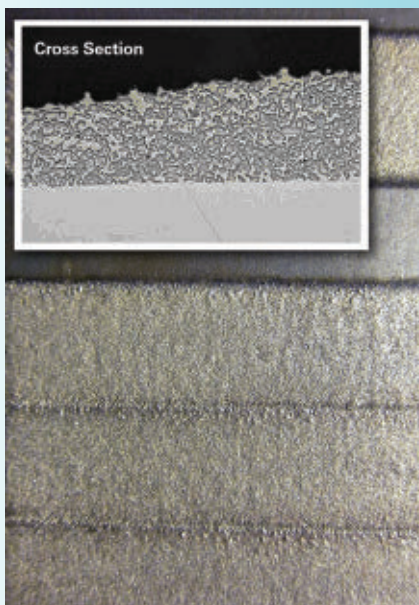
Figure 1. A large area, metallurgically bonded, thin (0.4 mm) clad deposit provided 2× better wear resistance in G65 wear tests against comparable thermal spray coating. A 1018 steel plate clad with 40 to 60 percent (NiWC powder with 60 percent WC). A 3 × 24 mm beam was used with 3 mm overlap to produce an effective clad width of 20 mm; 7kW and a process speed of 1.08 m/min was used to produce this sample part.
