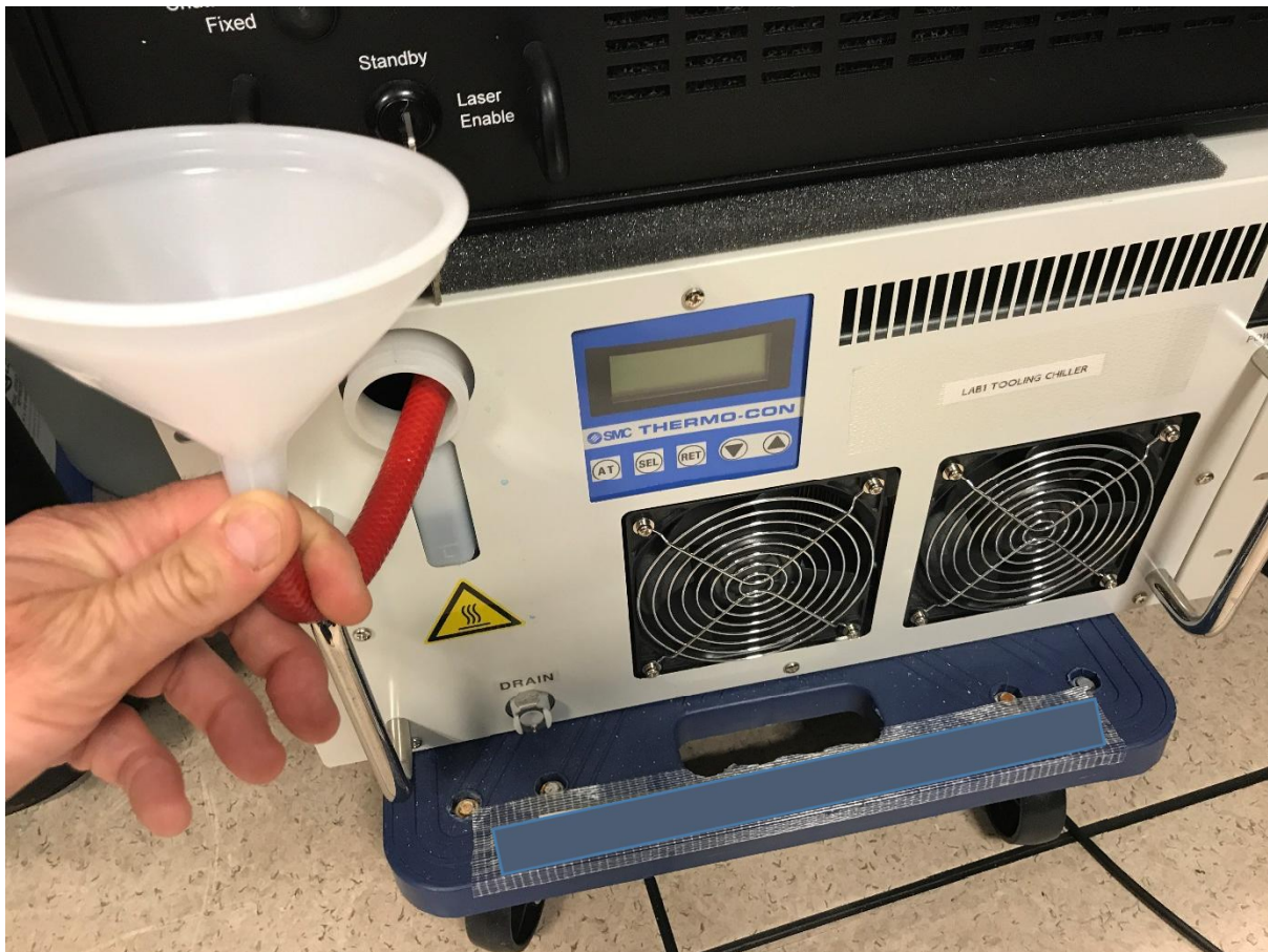
Fig 7. Photograph of Chiller refilling.
