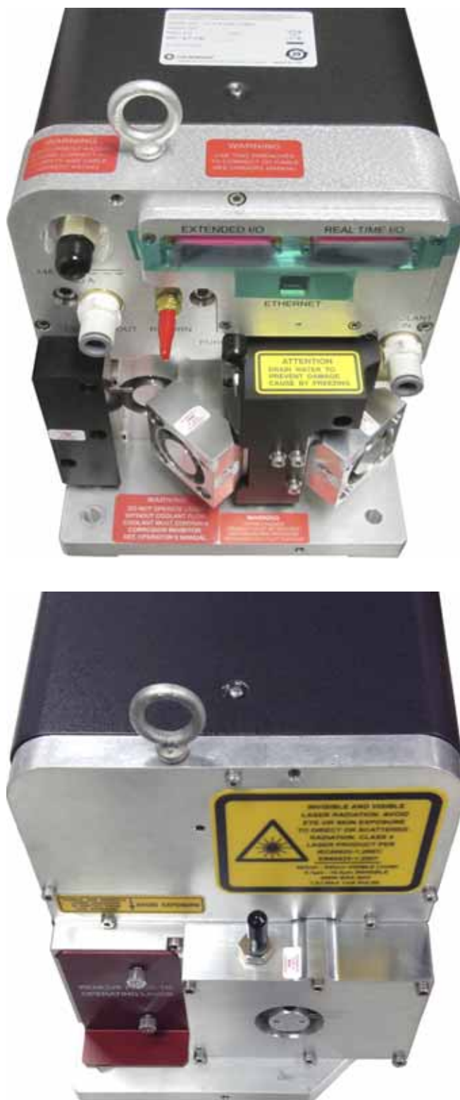
Figure 3-11. Eyebolts Installed in Laser System
