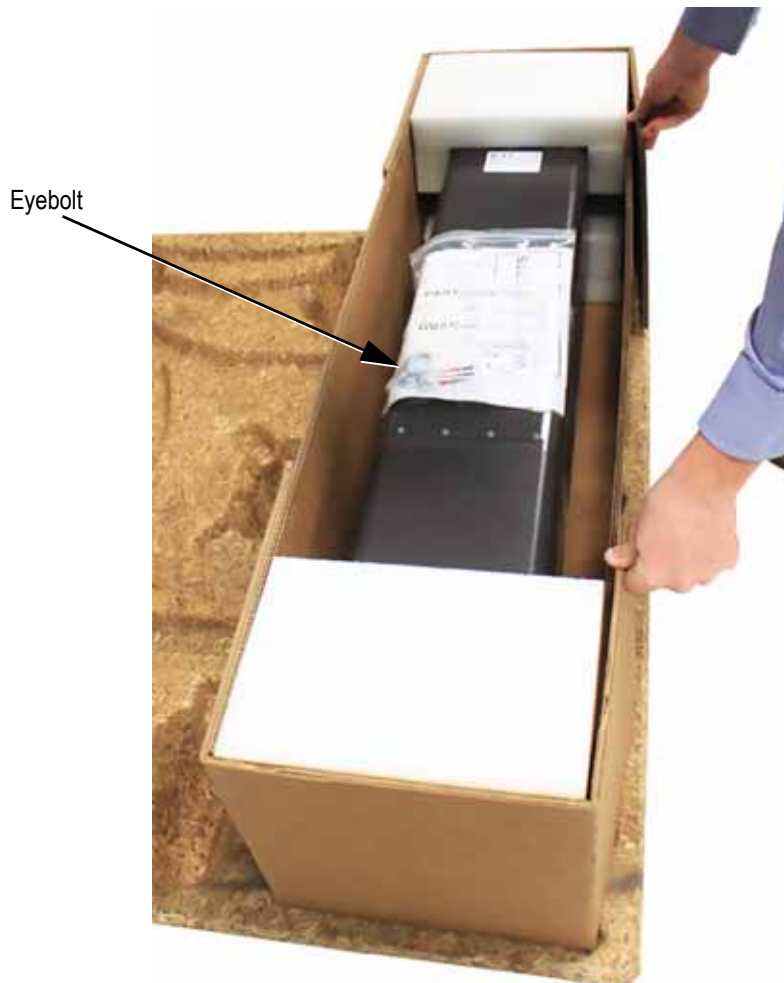
Figure 4-10. Removing the User Documents and Eyebolts
