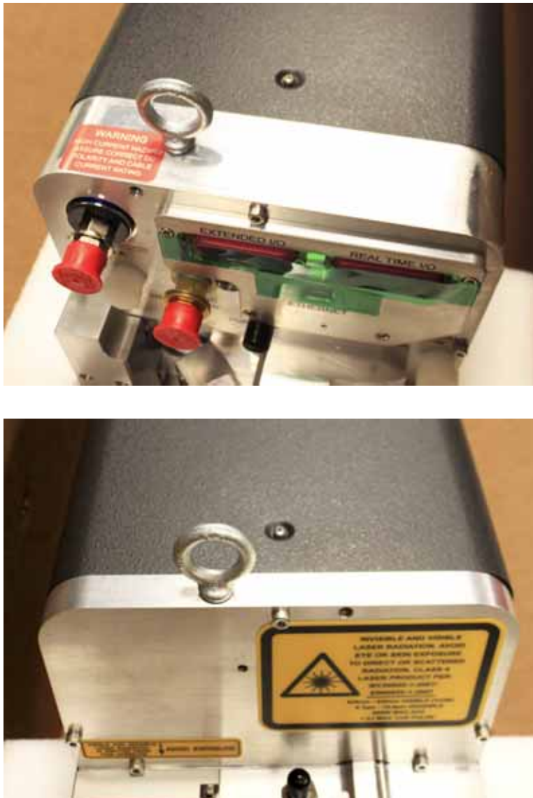
Figure 4-11. Eyebolts Installed in Laser System
