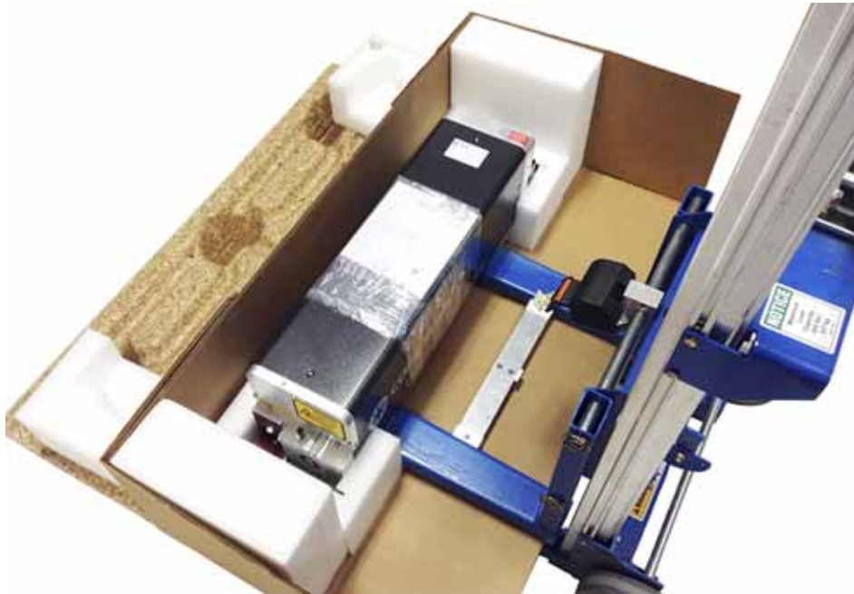
Figure 4-9. Lifting the Laser (J-2 and J-5 Series lasers shown as examples)
