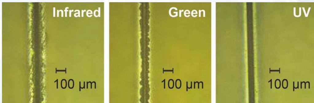
► Figure 3: A 220 µm thick simulated display layer on glass scribed with a Coherent HyperRapid NX laser with output in the infrared, green and ultraviolet. This clearly demonstrates the improvement in cut quality with decreasing wavelength. ►
