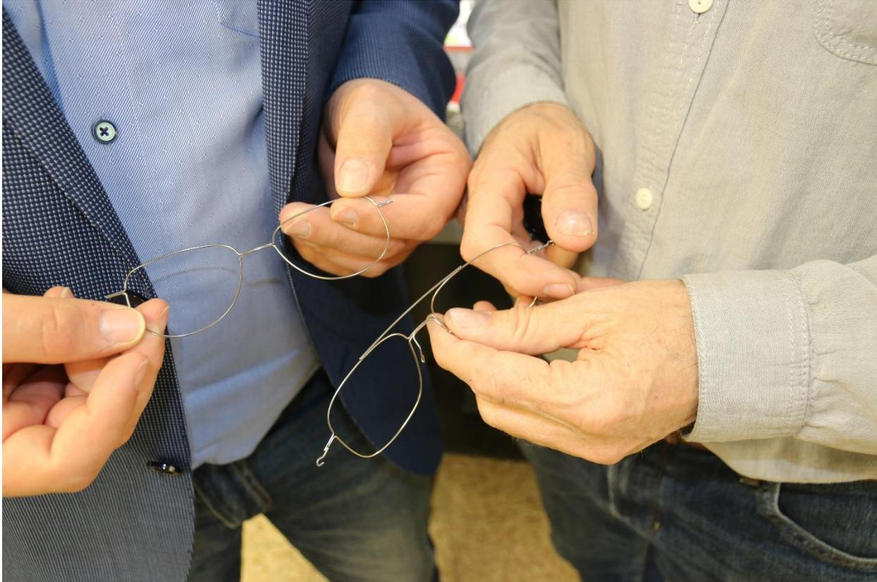
Glasses laser welded with the Coherent MPS Rotary system
