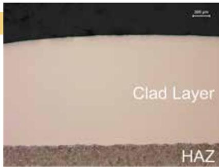
Figure 3. Cross section (etched in Nital) of a high power diode laser clad coating (Coherent HighLight operating at 4 kW). The heat affected zone (HAZ) is about 1 mm thick. This is much thinner than that obtained with other hard-facing techniques and indicates the lower heat input achieved with laser cladding.
