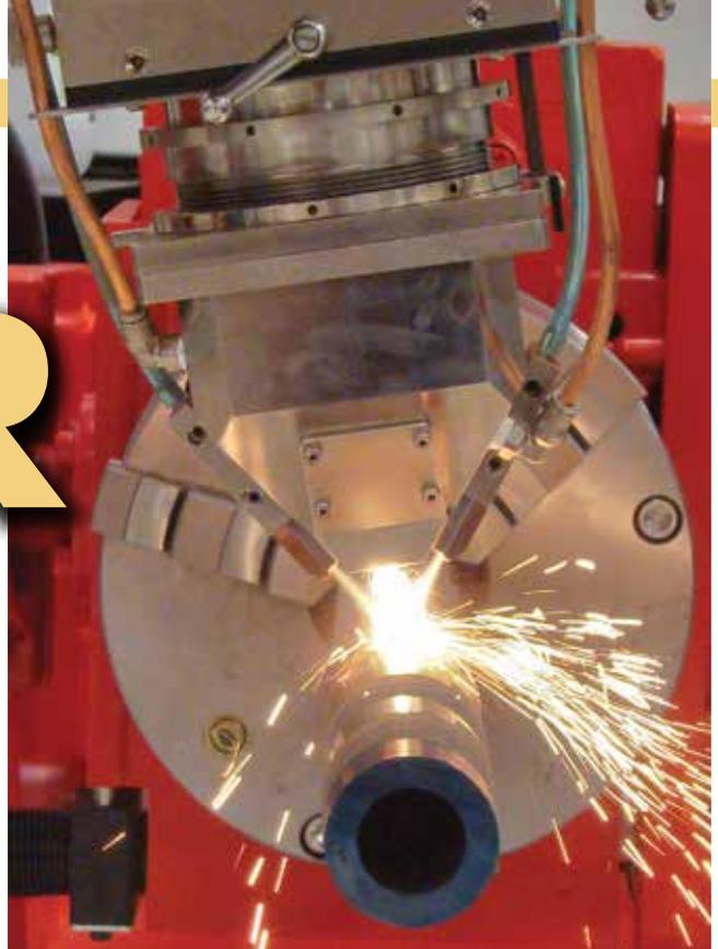
*A HighLight 8000D 8 kW high power direct-diode laser system performs large area laser cladding of Stellite 6 on flat and round low carbon steel materials.*
