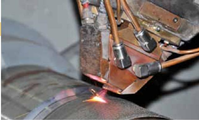
A high power direct diode laser is a compact assembly consisting of a very large number of lower power (about 100 W each) semiconductor laser emitters, whose output is combined into a single beam. Typically, this beam takes the form of a long, thin rectangle, usually around 3 mm wide, and anywhere from 6 mm to 36 mm long.
