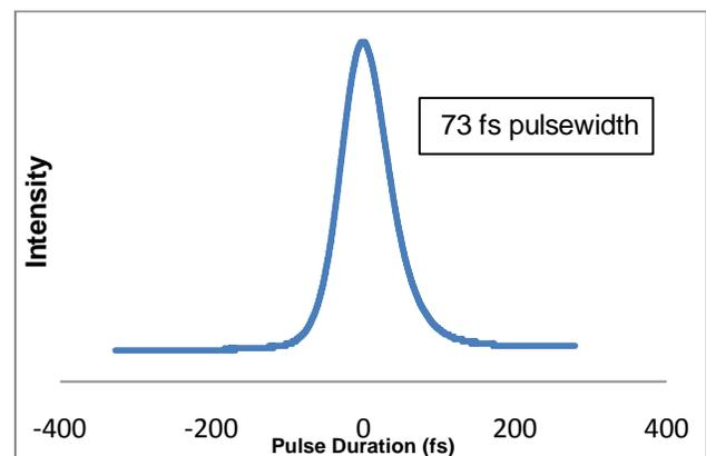
Figure 2, Autocorrelator trace showing 75 fs pulsewidth
