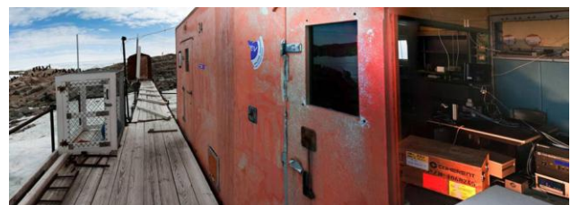
Figure 7. After a long multi-modal shipping journey to the French Antarctic base on the island of Dumont D’Urville, a Chameleon laser operated was successfully operated at a lab temperature of only 5 °C. Here it was used to make mode-locked CEAS measurements of trace atmospheric components at concentrations less than a part per trillion. Image courtesy of Thomas Paris, Dumont D’Urville Station, Antarctica.
