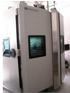
Figure 6. The HALT/HASS test chamber at Coherent.
