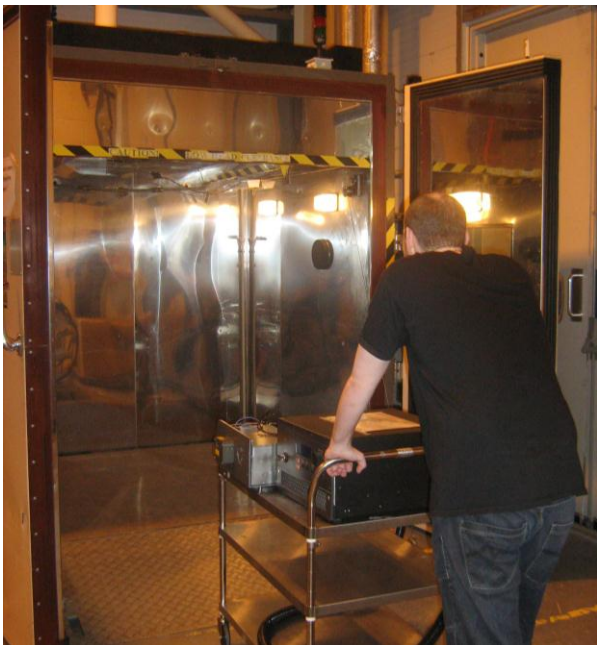
Figure 2 Chameleon being loaded into a temperature test oven
