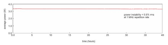
*Figure 6: Long term power stability of the White Dwarf operating at a pulse width of 8.6 fs and a 1 MHz repetition rate.*
