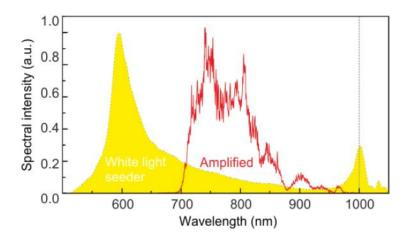
*Figure 4: The spectral profile of the WLG output and the amplified output from the OPA stage.*
