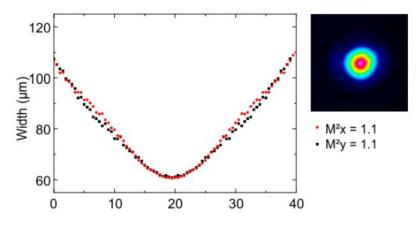
*Figure 7: The output is characterized by M2 values < 1.2 in both axes.*
