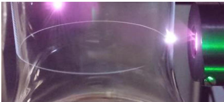
Figure 4: Coherent HyperRapid NX performing filamentation cutting on a wine glass.
