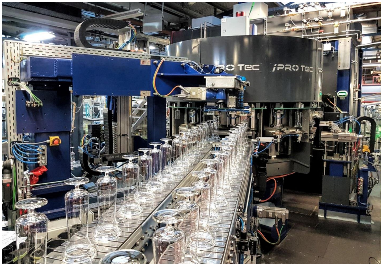
Figure 5: The IPROtec system is a fully automated machine for performing wine glass cap removal using SmartCleave at rates of up to 80 pieces/minute.
