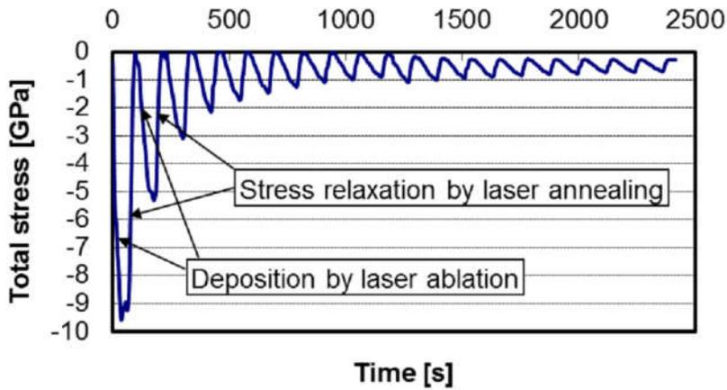
Fig 3: Total stress during the preparation of a 1  $\mu\text{m}$  thick ta-C film on a 400  $\mu\text{m}$  thick silicon substrate, produced by successive deposition and annealing at an ablation fluence of 12  $\text{J}/\text{cm}^2$  and an annealing fluence of 150  $\text{mJ}/\text{cm}^2$ .
