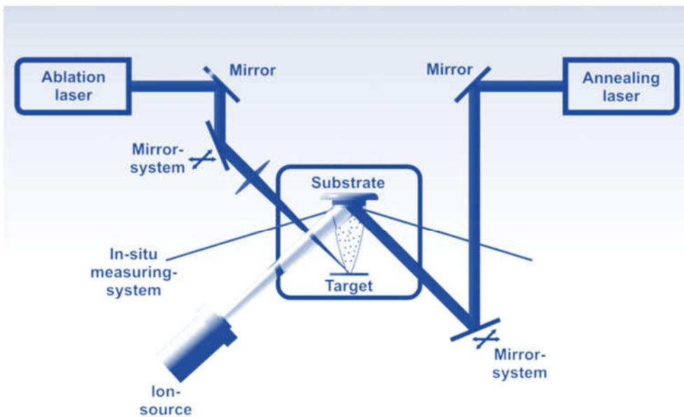
Fig. 1: Schematic of the experimental set-up used for the preparation of stress-free, ta-C films.
