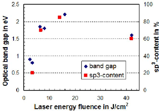
Fig 2: The  $sp^3$ -content and optical energy band gap of PLD grown ta-C films as a function of laser fluence.
