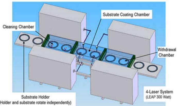
Fig 4: Concept of a continuous DLC coating system based on four high power excimer lasers.
