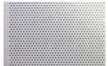
Fine Hole Drilling
